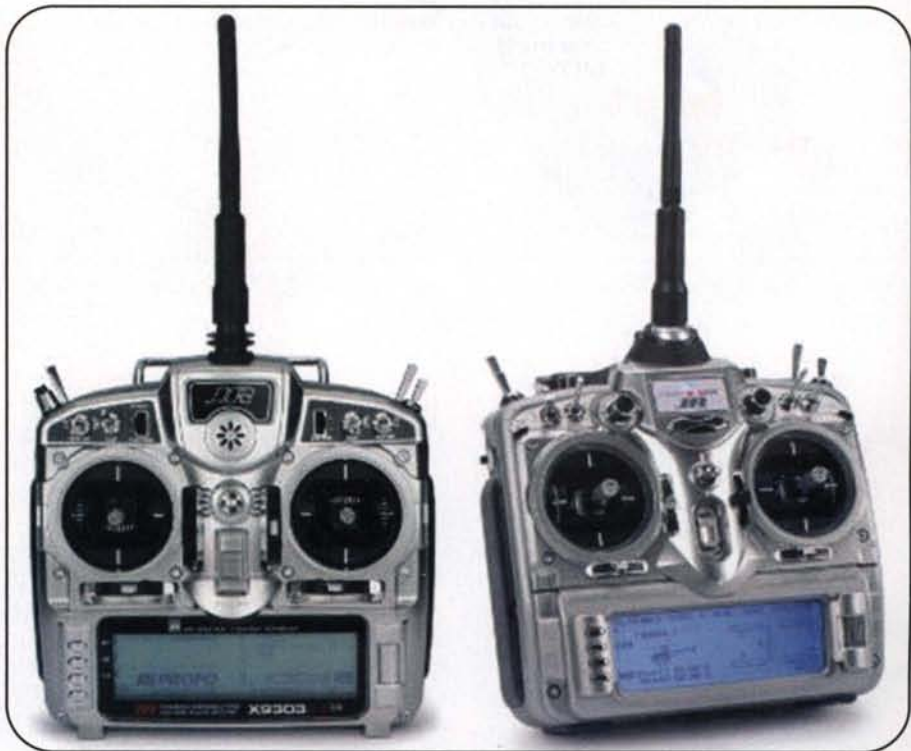
Module-equipped JR transmitters available for 2.4 GHz, 50 MHz, or 72 MHz.
