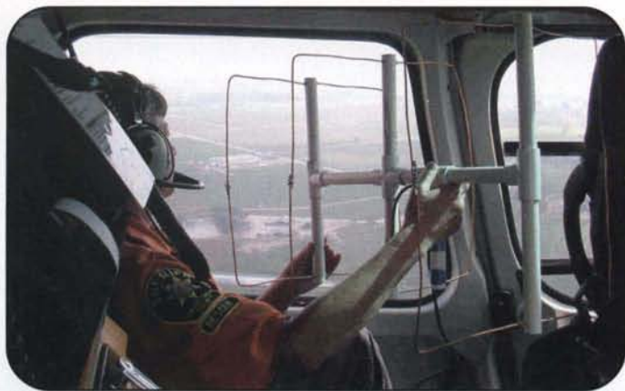
Eve Vigil, KF6NEV, gets airborne bearings with a home-built 215-MHz cubical quad. Compared to an equivalent Yagi, she found that it is better performing and easier to use in the helicopter. (Photo courtesy of WA6NGH)
