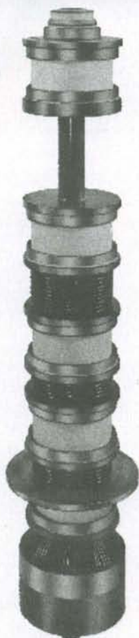
Photo B. The Eimac 3K2500LX Klystron used for early moonbounce work.
