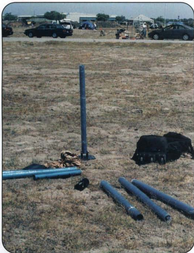
Photo B. The BlueSky Lite mast sections slip together and lock in place in seconds. (WB6NOA photo)
