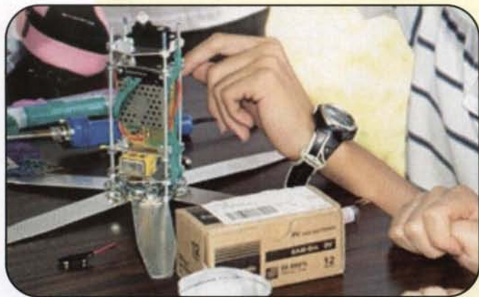
The electronics inside one of the cansats.
