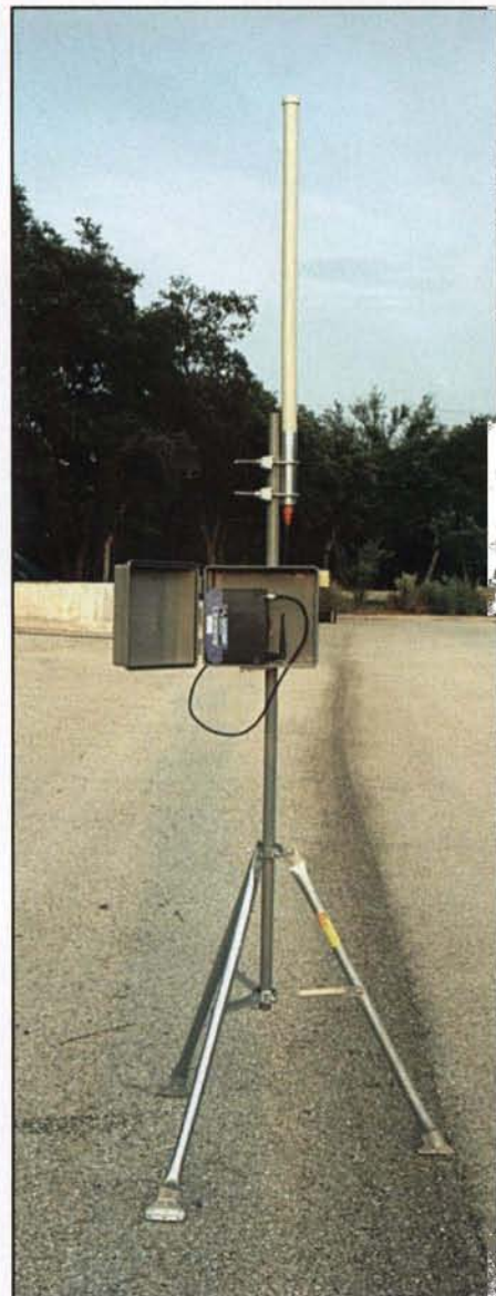
Photo C. This is typical stand-alone, omni-directional, fully automatic HSMM-MESH® node. (Photo credit David B. Rivenburg, AD500)
