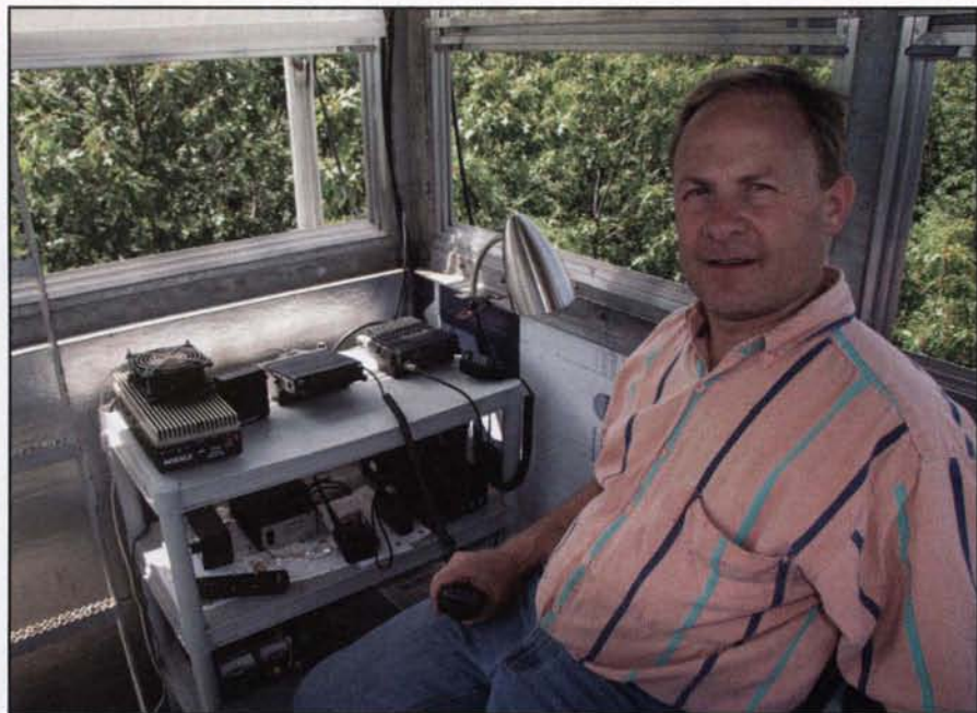
Photo 7. John's station consists of a 2m/440MHz Yaesu FT-8800 matched with a 160-watt Prodigy Amp and a 220 Alinco DR-235MKIII coupled with a Mirage 1012 amp, 120 watts. Either can be mated to a West Mountain Radio CLR DSP audio processor.
