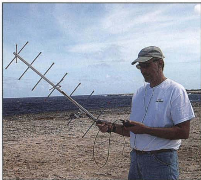
Photo 10. The FM OSCAR satellites can be worked using an HT and a handheld Yagi antenna.
