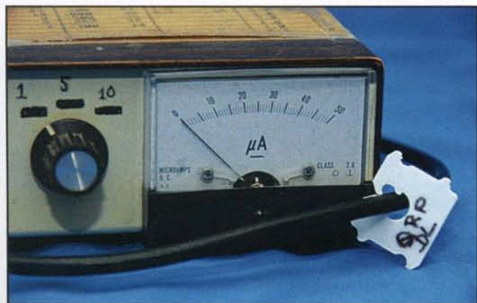
Photo 3. A plastic tag on the coaxial cable for my QRP wattmeter. This is a very inexpensive way to assure that you can easily identify all the cables in your shack at a glance.
