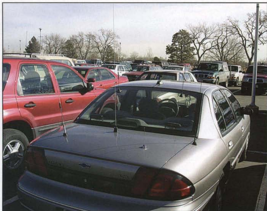
Photo 4. This sedan has a good collection of VHF/UHF vertical antennas installed. A good mobile installation makes for a fun road trip, but you can probably do just fine with fewer antennas than this.
