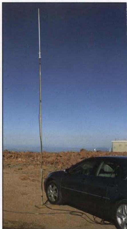
Photo 6. The vertical 2m/70cm antenna is attached to a mast using a "drive on" mount.
