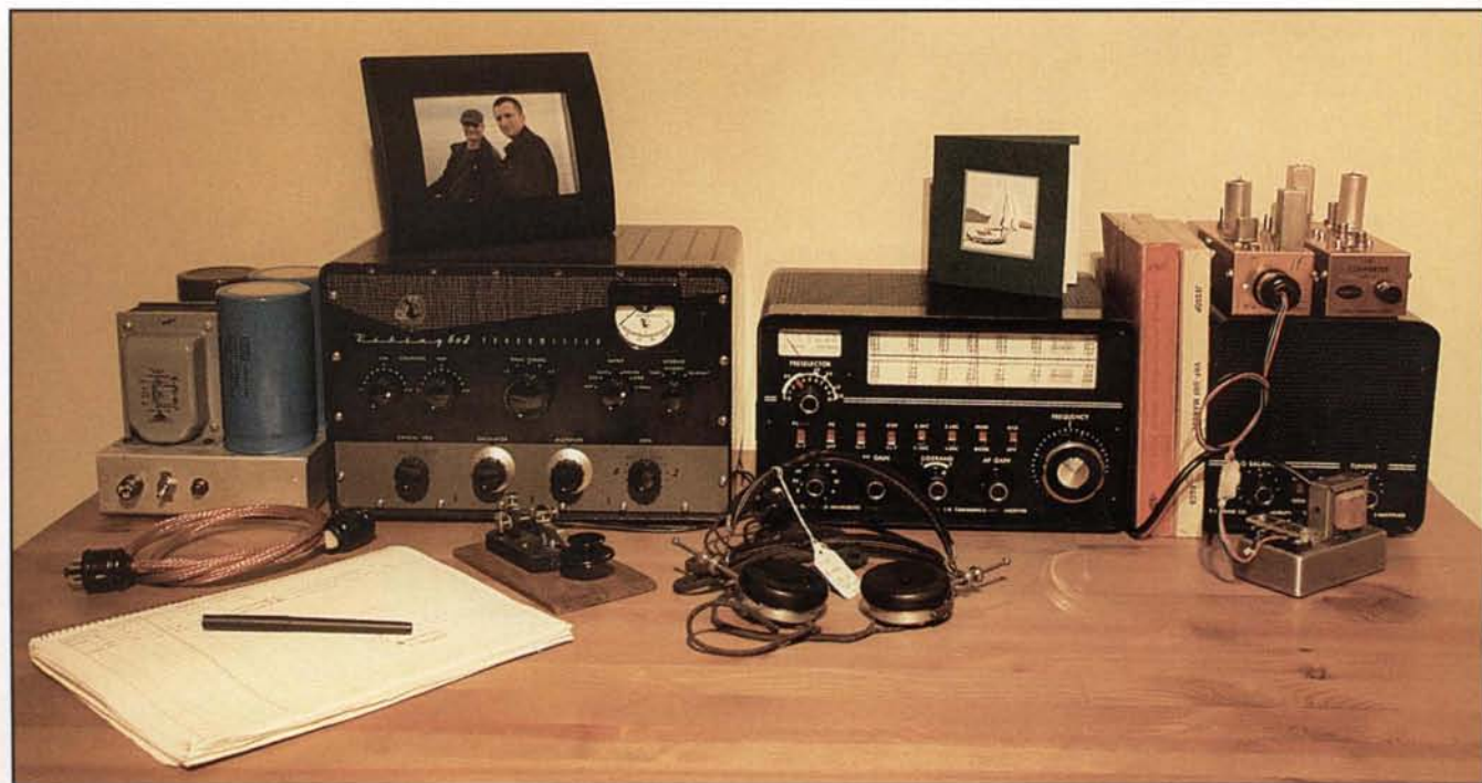
Photo 1. An historic VHF experimenter's station. From left to right are a home-built power supply, Johnson 6N2 transmitter, Drake 2A tunable IF receiver, and a pair of Ameco 6- and 2-meter Nuvistor converters sitting on top of the Drake 2AQ speaker Q-multiplier. (Photos courtesy of the author)
