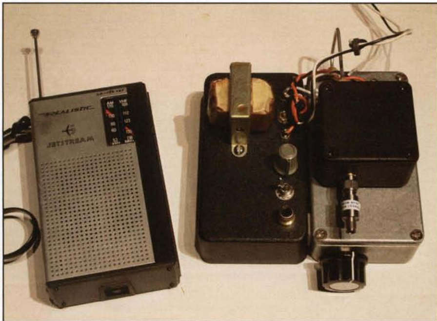
Photo 2. A complete low-power, 2-meter AM station using the 2-meter AM transmitter described in the last issue of this magazine and a modified portable AM aircraft receiver from the bargain table at the local RadioShack.
