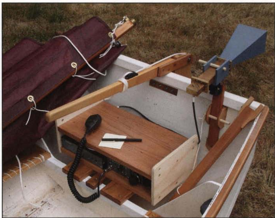
Photo 7. A 5.8-GHz microwave station mounted in the stern of the sailboat for experiments with W7YOZ along Pickering Passage in Washington State.
