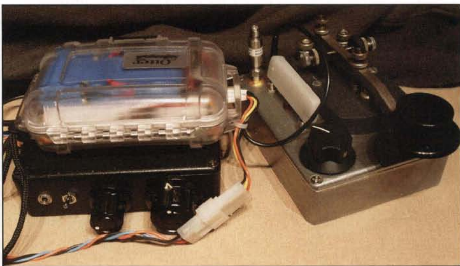
Photo 6. A serious 6-meter CW station optimized for use in the boat. The handheld CW transmitter includes the key on top and batteries inside. The long white plastic lever is the T-R switch, operated by thumb. The receiver is the Rcx1 and microR2 from Kanga US. The receiver battery pack and converter are in an Otter waterproof plastic box from REI.
