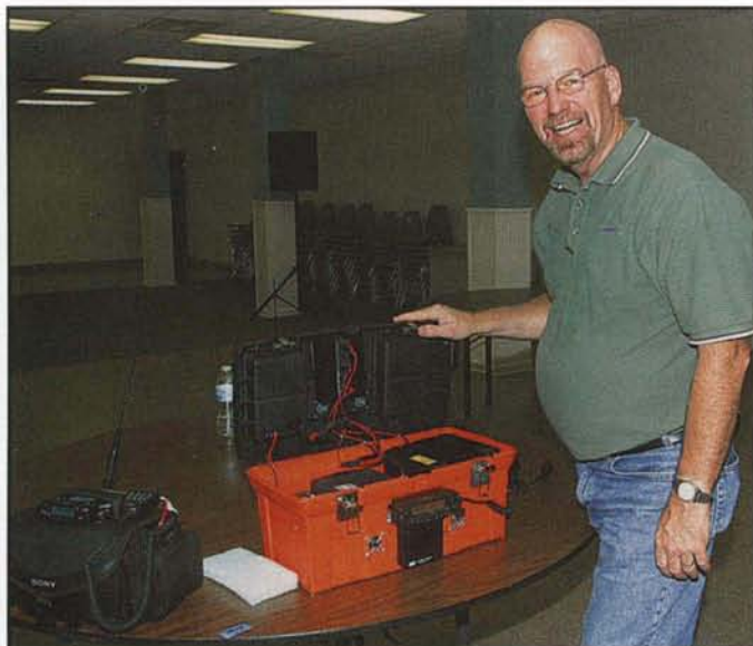
David Adcock, KA4KKF, one of the "technical heavies" of the Gwinnett ARES group, has a small tool kit pressed into service for his Go-Kit. The kit contains a dual-band VHF/UHF radio, power supply, and packet radio gear for a portable FM voice and 1200-baud VHF packet station.
