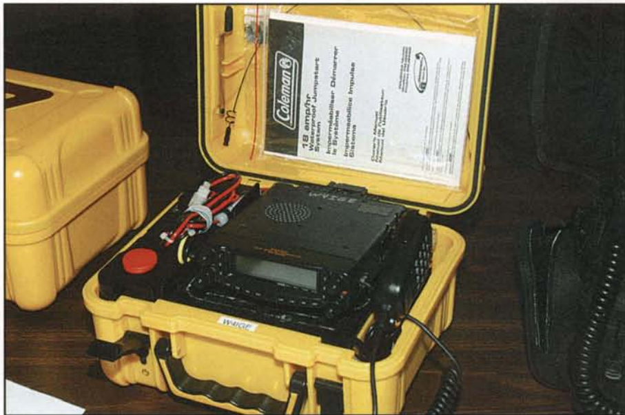
One of two Go-Boxes by Hal Collier, W4IGE. This is Hal's FM voice kit consisting of a dual-band VHF/UHF FM transceiver, 17-amp/hour battery supply, mic, and portable antenna. His other box (identical to this one) has a 2-meter rig and packet radio TNC for his portable packet station.
