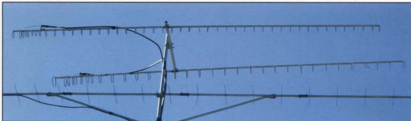
Photo A. Loop Yagis, which are electrically similar to cubical quads.
