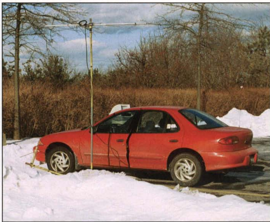
Photo 3. A January 2003 VHF contest QRP effort with a 1998 Chevy Cavalier using a three-element 6-meter Yagi.
