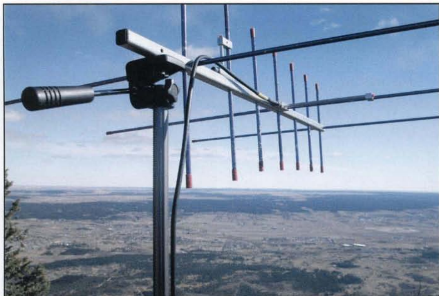
Photo 5. The Arrow II antenna is a Yagi that works on 2 meters and 70 cm.
