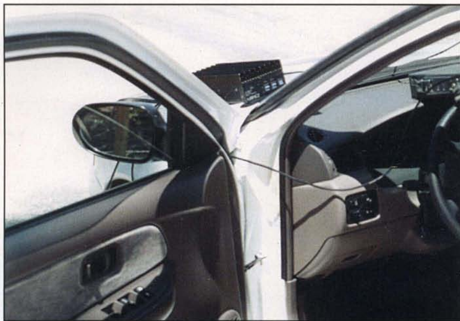
Photo 6. Also during the author's rover effort in Wyoming and Colorado for the June 1996 VHF contest, this is the inside of the car with the FT-690 on the dashboard and the Mirage 1015A amplifier on the hood of the car.
