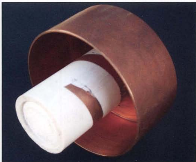
Photo 3. Short helix for use as a dish feed.
