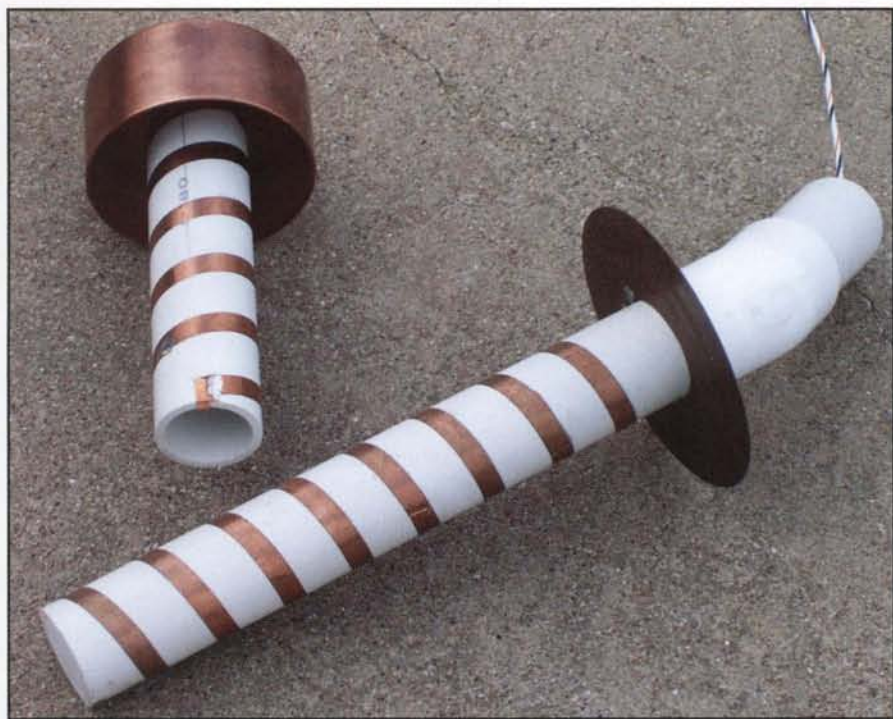
Photo 4. More helix antennas wound on plastic pipe.
