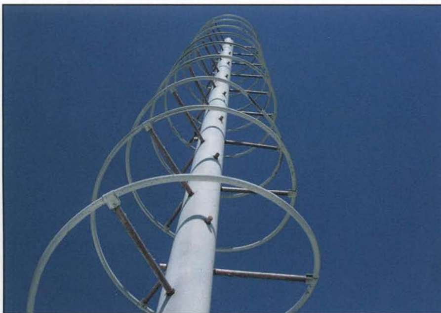
Photo 7. A helix antenna the way NASA likes them.
