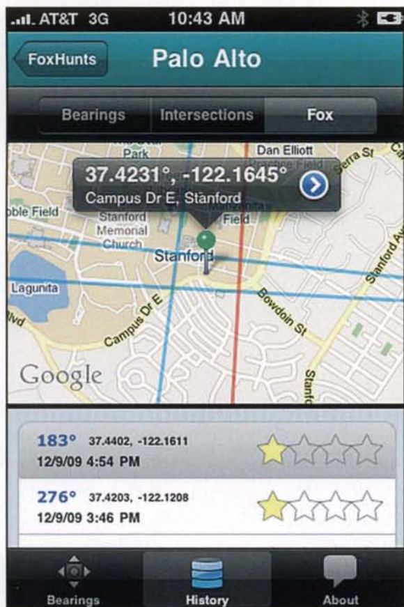
Triangulated bearings on the screen of an iPhone with the FoxHunt™ application. There are four bearings; the selected one is red. The program makes a best estimate of the fox location (the green pushpin), based on the confidence level given to each bearing.
