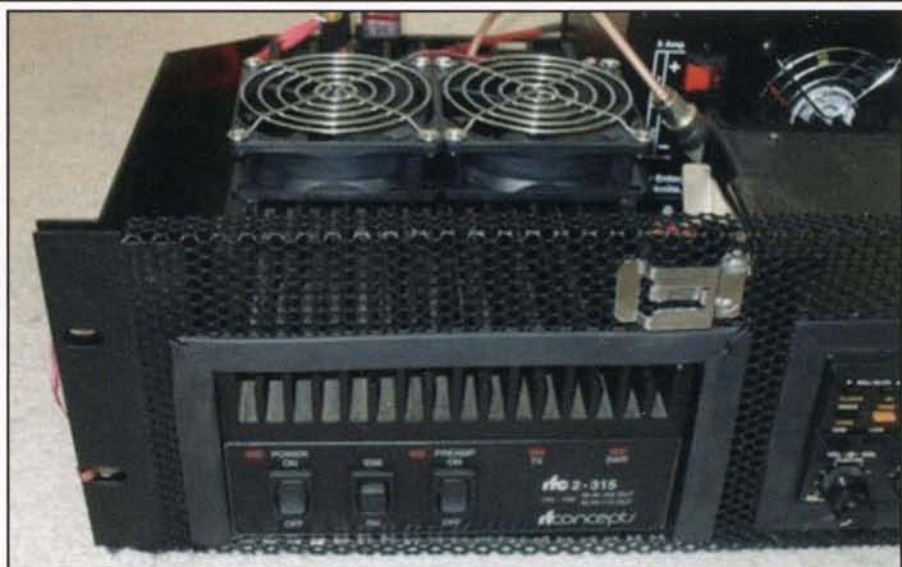
Photo 5. The amplifier and cooling fans.
