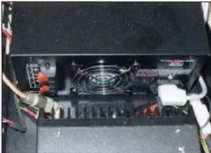
Photo 6. The power supply is positioned so its cooling fan also cools the radio's heatsink.
