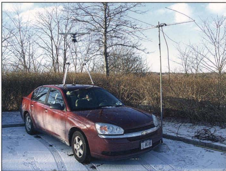
Photo 8. This is the current antenna setup that has been used by the author for his QRP portable setup since January 2007. The three-element 6-meter Yagi is on an umbrella stand, while the three-element 2-meter Yagi is mounted on a tripod situated on the roof of the car with the latter antenna also used on 432 MHz, mainly for simplicity. There is a mag-mount vertical located underneath the tripod which is used for 220-MHz FM.
