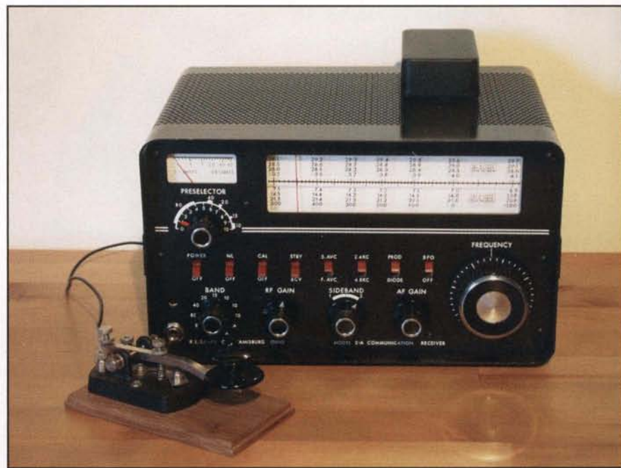
Photo 3. For extra shielding, put the Rcx1 in a diecast box. This is a very capable 6-meter weak-signal receiver using the new Rcx1 and a vintage Drake 2A.
