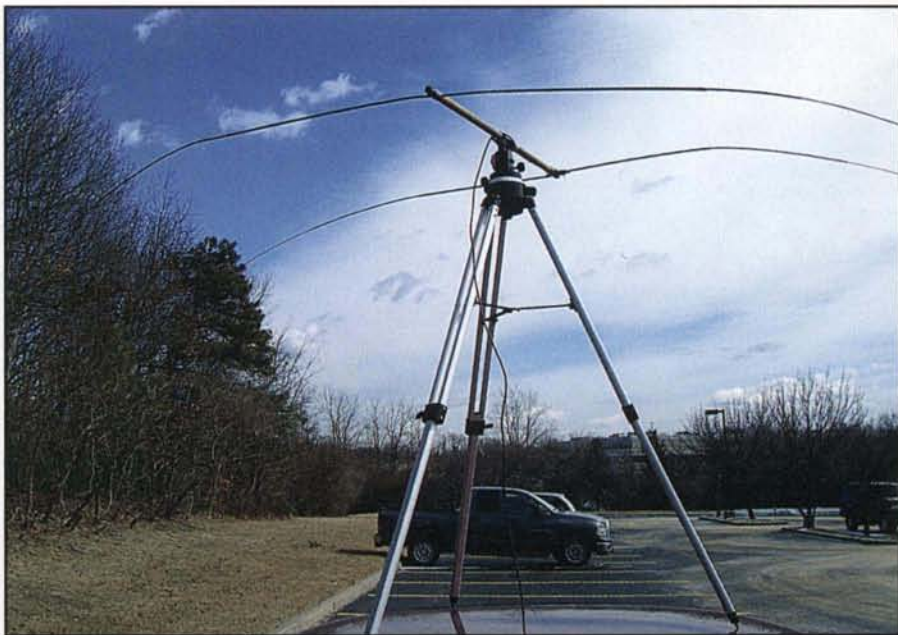
Photo D. Here is the same telescoping tripod used to now mount a 2-element 6-meter Yagi on top of the author's car at one of his work locations a few years ago. This setup was suitable enough to work stateside stations via sporadic-E as well as some DX into Europe, with Italy being worked in June 2006.
