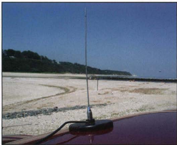
Photo A. This 1/4-wave vertical for 222 MHz is a simple antenna that is a baseline and takes the least amount of effort to set up. Different length antennas for 6 meters, 2 meters, and 432 MHz can also be used on the same mount through the use of an Allen key on the mounting piece. (Photos by the author)
