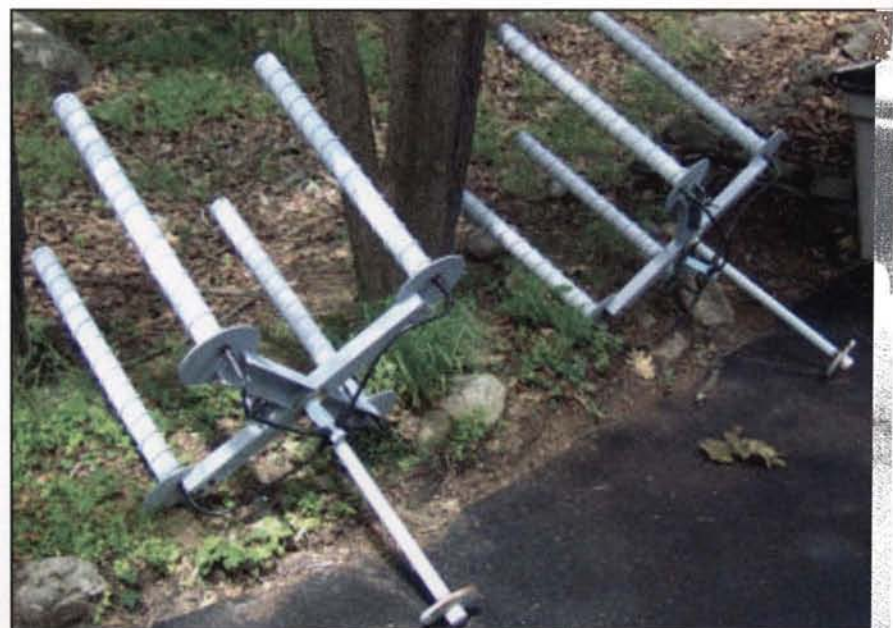
Photo B. Helix array removed from service to make way for new loop Yagis.
