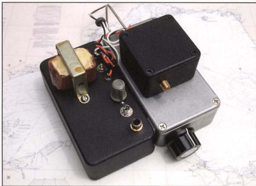
Photo D. After the experiments, the next step is to package the transmitter in a convenient form. This version is a 100-mW carrier or 400-mW PEP 2-meter AM transmitter using a 144-MHz VHF signal source, a simple two-stage class C RF amplifier, the audio amplifier from an R2pro kit, and a small transformer. The total DC power drain from the AA cell pack is less than needed to power the author's 10-mW SSB exciter. Below 1 watt output, AM can be more efficient to generate than SSB.
