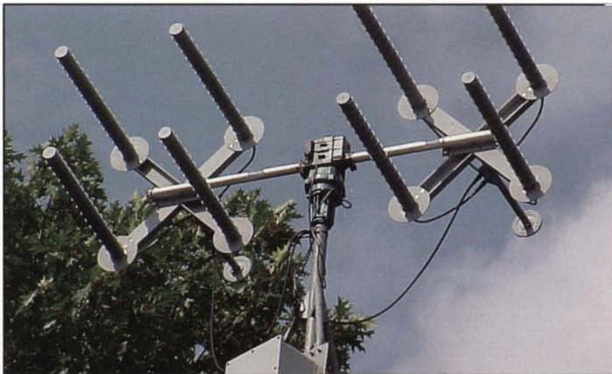
Photo A. Original helix array at the W2ETI EME Beacon.
