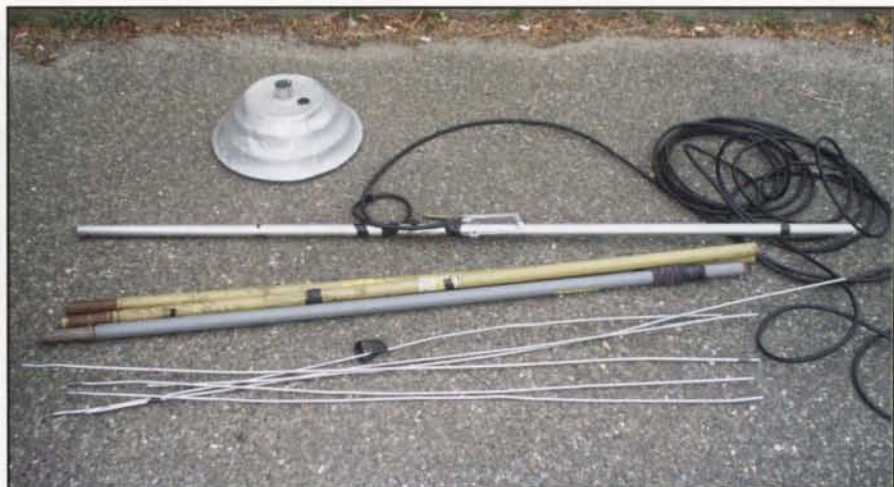
Photo E. The 6-meter setup that the author uses for his portable operations during VHF contests and other events. There is an umbrella stand with concrete added, the 3-element 6-meter Yagi, three 5-foot mast sections, and the six elements for the Yagi. Mast sections can be found at RadioShack, but some catalog searches may be required. Newer mast sections are painted in gray compared to yellow used in the past.
