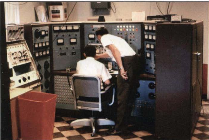
Photo I. The controls for the 430-MHz klystron transmitter, with power levels of 2.5 mW peak, 150 kW average.
