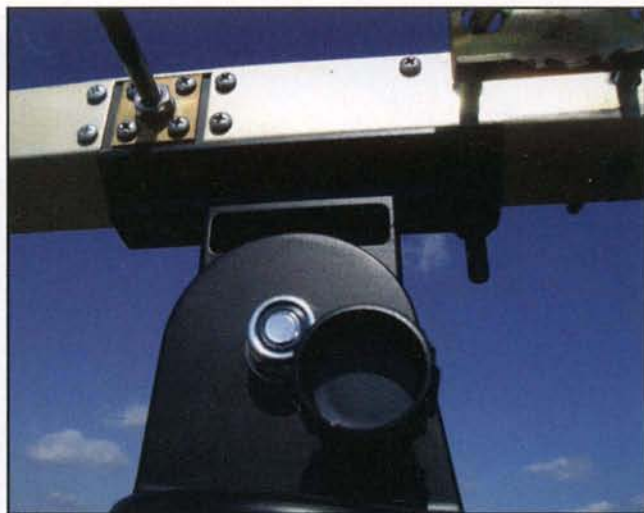
Photo C. This closeup shows how the antenna can fit into the telescoping attachment of the tripod using bolts through the telescoping bracket. The author has yet to use this tripod for its intended use over the four years he has owned it.
