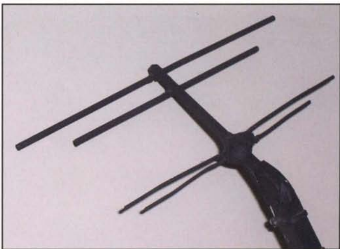
Photo B. Close-up of the 902/1296 MHz feed.
