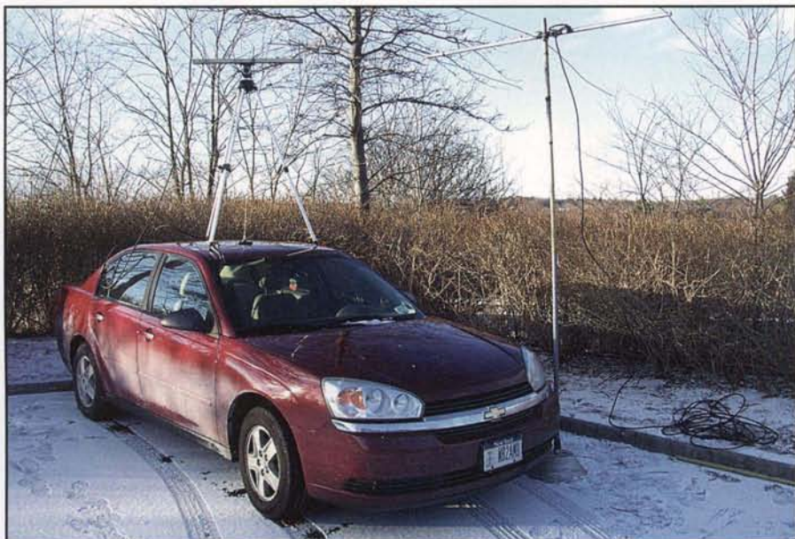
Photo G. This photo shows the three different portable antennas described in this article: the 220-MHz vertical positioned on the car roof, a 3-element 2-meter beam on a tripod positioned on the car roof, and the 6-meter beam mounted on mast sections off to the side of the car (at 10 feet in height due to strong winds that were present at the time in Long Island during the January 2010 VHF contest).
