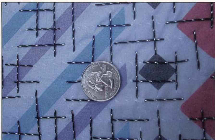
Photo B. One thing that is important is the spacing between parallel threads. The highest frequency I wanted to use was 2.4 GHz, so this works out to about half an inch between threads. Have some metallic thread about every half-inch that goes vertically and horizontally.
