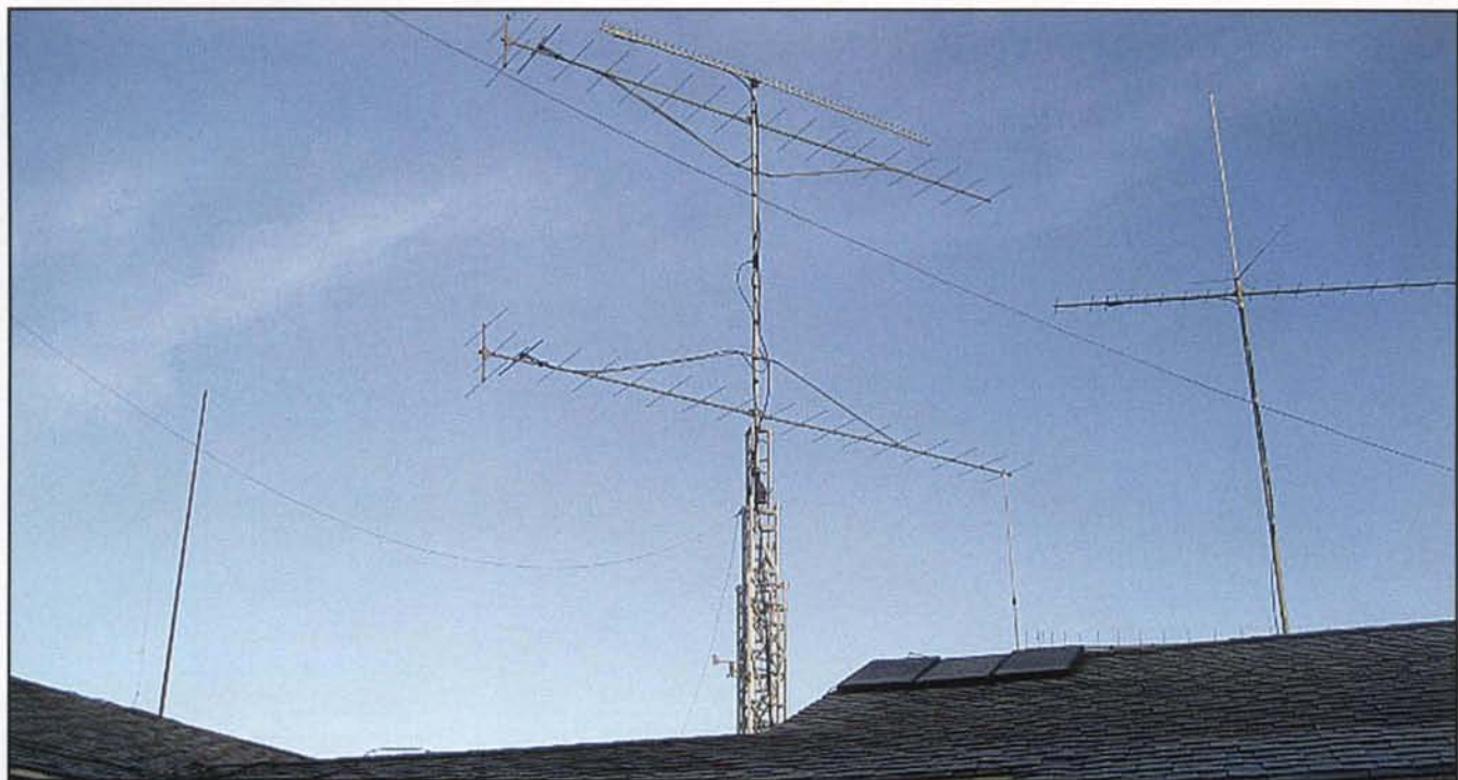
The author listens for tropo from Hawaii using this stack of 144-MHz long boomers. Topping the boomers is a 1296-MHz loop.
