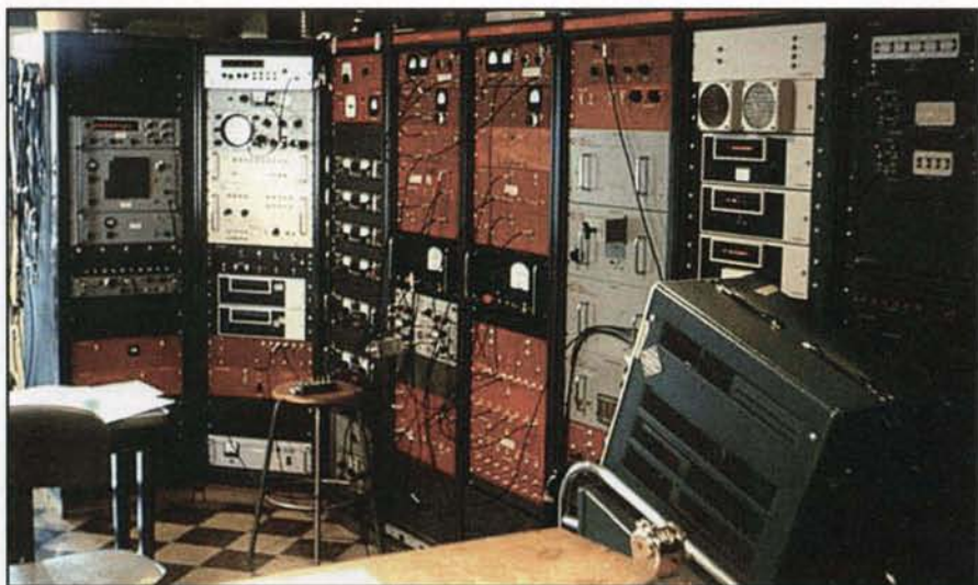
Photo H. Some of the equipment used in the receiver room, with the master clock and frequency standards.
