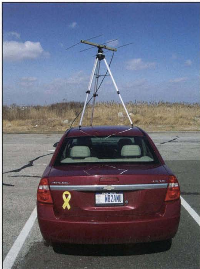
Photo B. This photo shows the use of a telescoping tripod to mount a 3-element 2-meter Yagi on top of the author's car. This setup is good when the portable arrangement is in the middle of open space with no trees or other support available.
