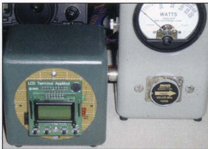
Figures 1 & 2. The digital wattmeter element is designed to either replace the analog meter element inside the Bird Wattmeter (left) or be mounted in an external enclosure to augment the standard Bird (below).
