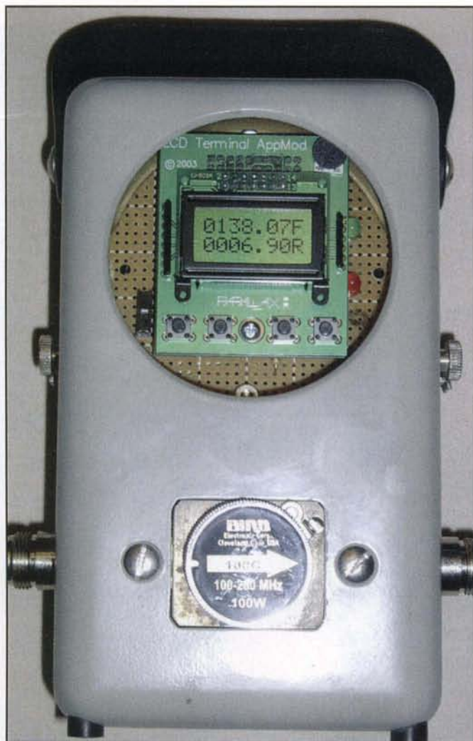
Figures 1 & 2. The digital wattmeter element is designed to either replace the analog meter element inside the Bird Wattmeter (left) or be mounted in an external enclosure to augment the standard Bird (below).
