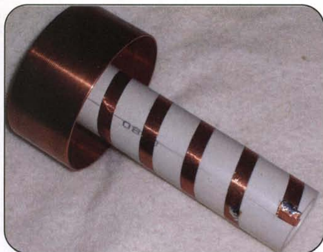
Photo B. Pitfalls when constructing helix antennas.
