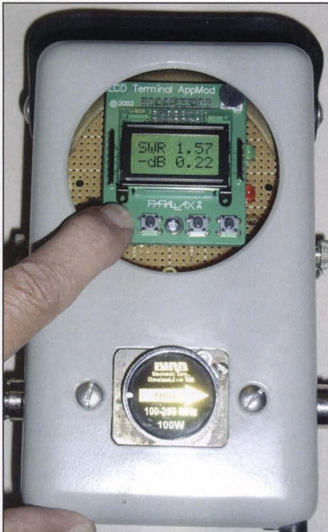
Figure 7. While applying power to the wattmeter, press button 1 to calculate the VSWR and power loss. The top line of the LCD will display the SWR and the second line will display the power loss in dB.
