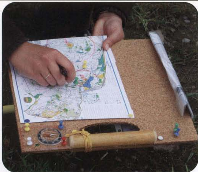
At the 2009 USA and Region 2 ARDF Championships near Boston, Susanne Walz, DG4SFF, of Germany used this board and pushpins to keep track of her bearings and her position on the map while out on the courses. (Photo by Joe Moell, KØOV)
