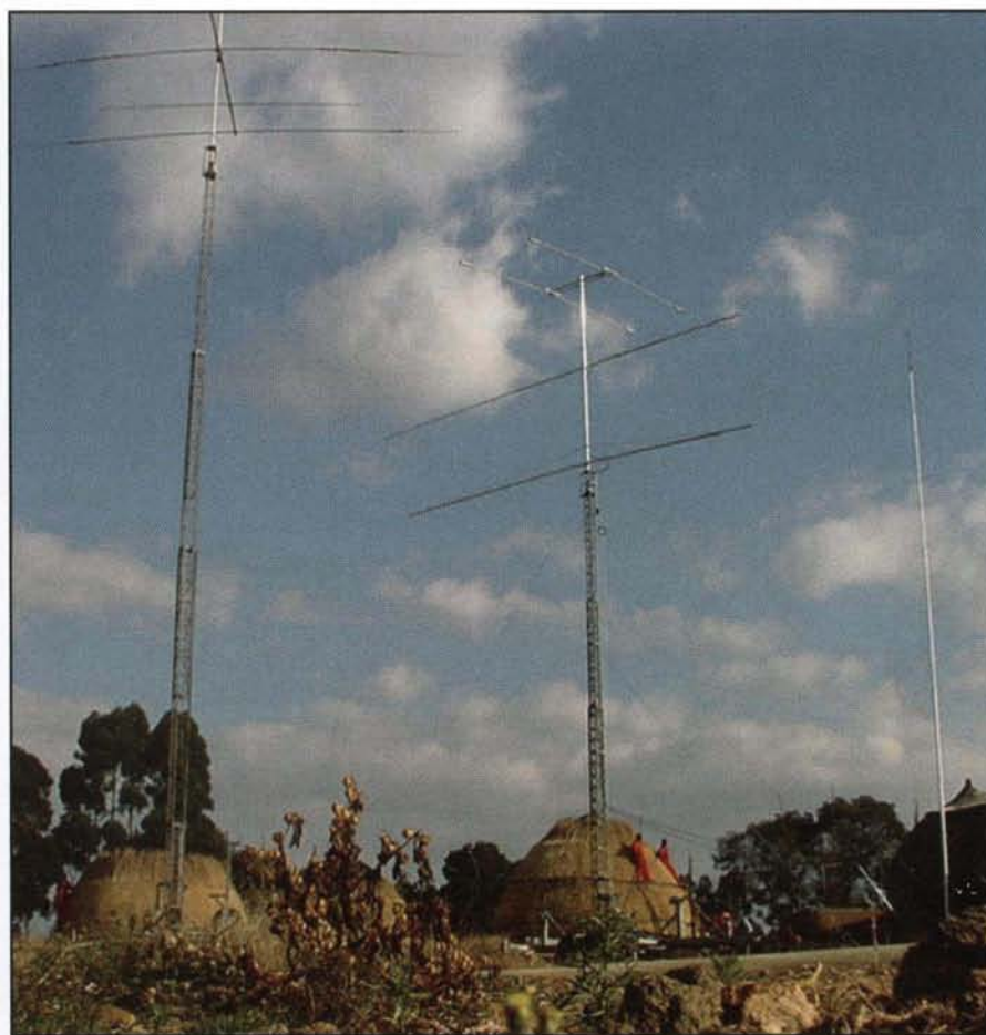
Photo C. 3DAØJR Swaziland (op: ZS5JR) HF + 2-meter EME station, KG53ms, July 2005. One Yagi on azimuth rotor.
