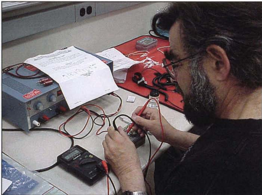
Astrophysicist Malcolm I. Raff, WA2UNP (SK), assembling and testing a low-noise preamplifier at The SETI League's 2003 technical symposium. Mal's amplifier did not oscillate! (N6TX photo)
