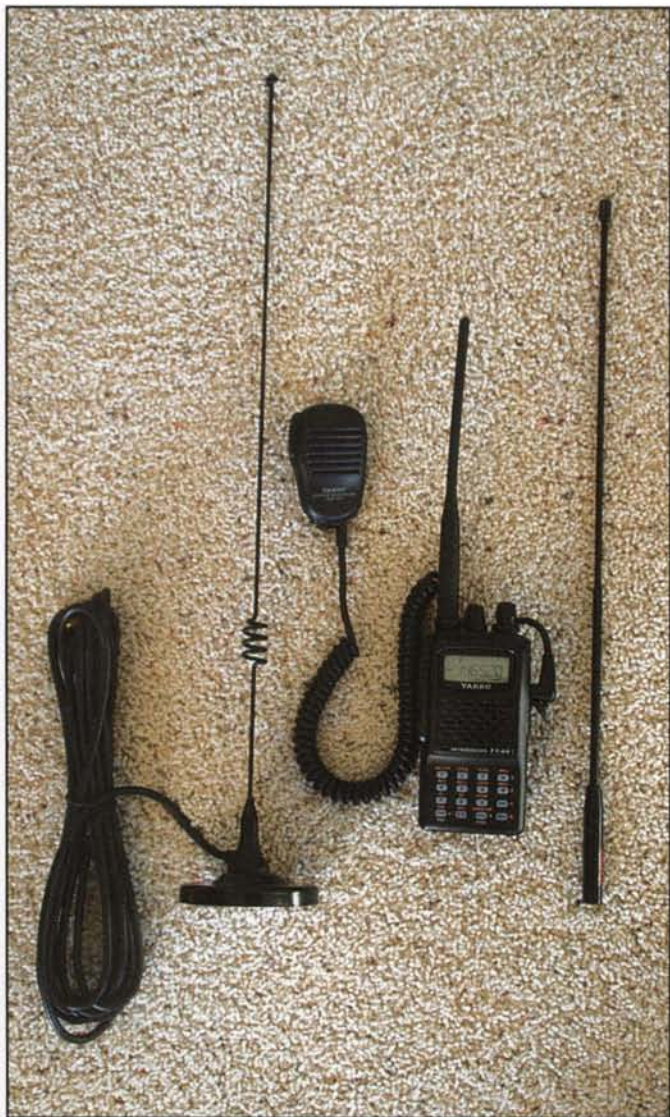
Photo 2. A handheld radio is shown here with a standard rubber-duck antenna. To the right is an extended-length portable antenna and to the left is a compact magnetic-mount mobile antenna.
