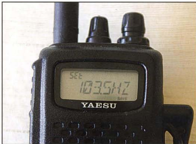
Photo 3. Most modern FM transceivers allow the CTCSS tone to be set by the front-panel controls and stored in memory.
