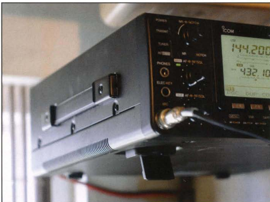
The ICOM IC-9100 is easy to move around with its handle and rubber feet. (Photos by the author)
