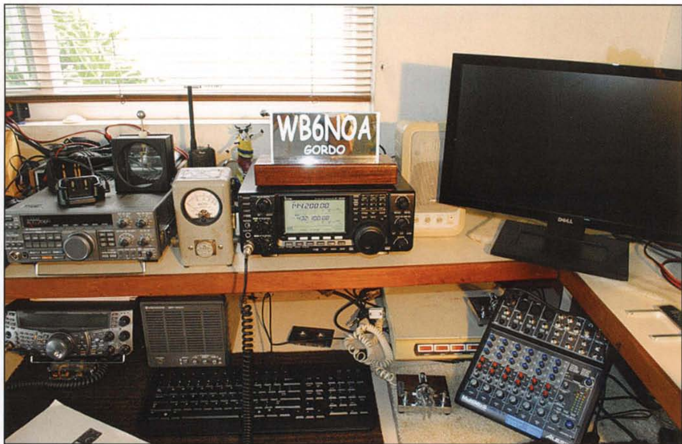
The new ICOM IC-9100 takes a place of prominence at the WB6NOA amateur radio station.
