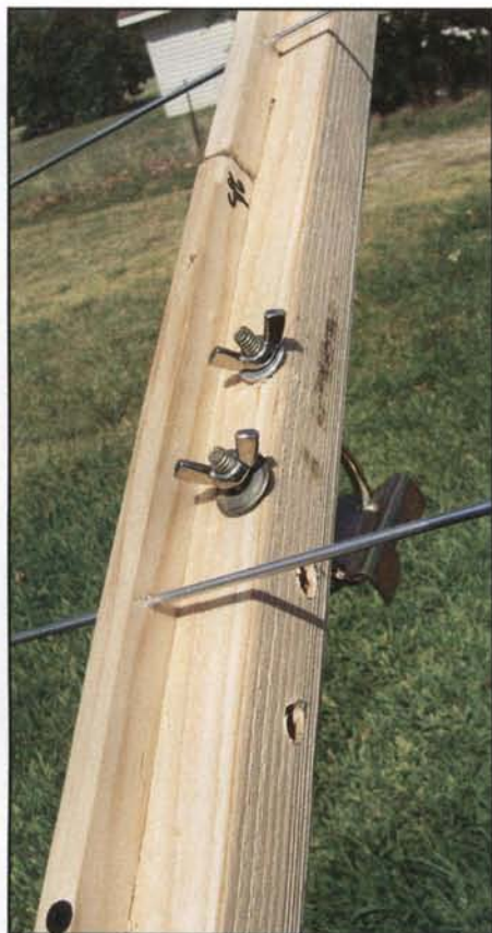
Photo 4. Support boom and mounting.
