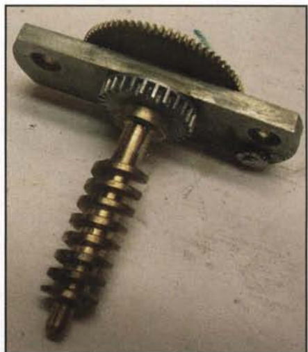
Photo 18. The worm gear after removal of the gear shaft.
