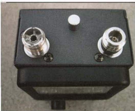
CAA500_top: The CAA-500 utilizes a high-quality "Type N" connector above 300 MHz, to ensure accuracy of SWR measurements relative to 50 Ohms in the UHF range.
