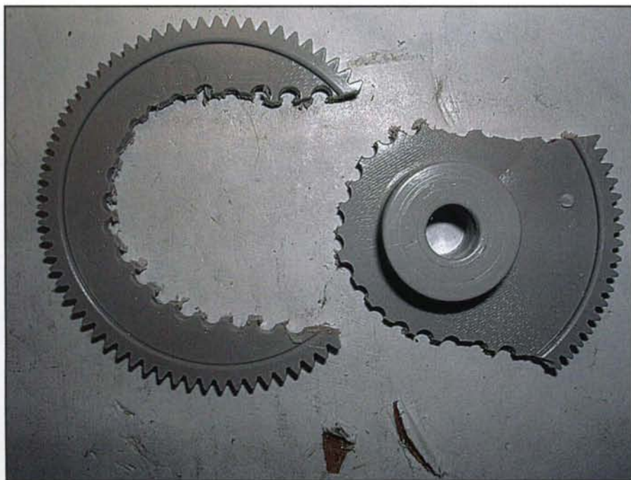
Photo 7. The large plastic gear that goes in the EL rotator. It shows how to begin forming the slot so that it can be mounted on the rotator collar. Be sure to stay completely inside the scribe marks.
