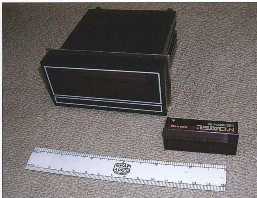
Photo 2. The panel meter on the left has an open-frame power transformer—bad news for the sensitive circuitry close by. Use one similar to the one on the right, as it keeps the size of the cabinet small.
