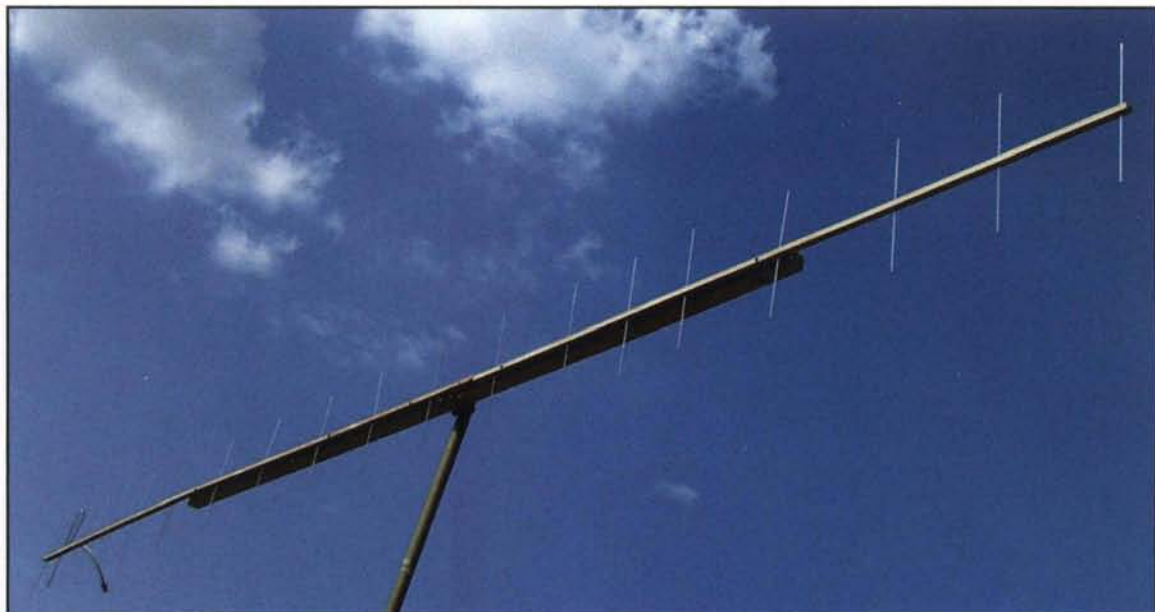
Photo 3. Twenty-element 432-MHz Yagi.
