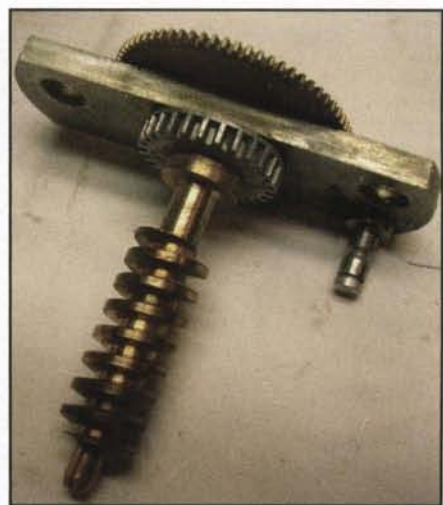
Photo 17. The stock worm gear before the gear shaft has been removed.
