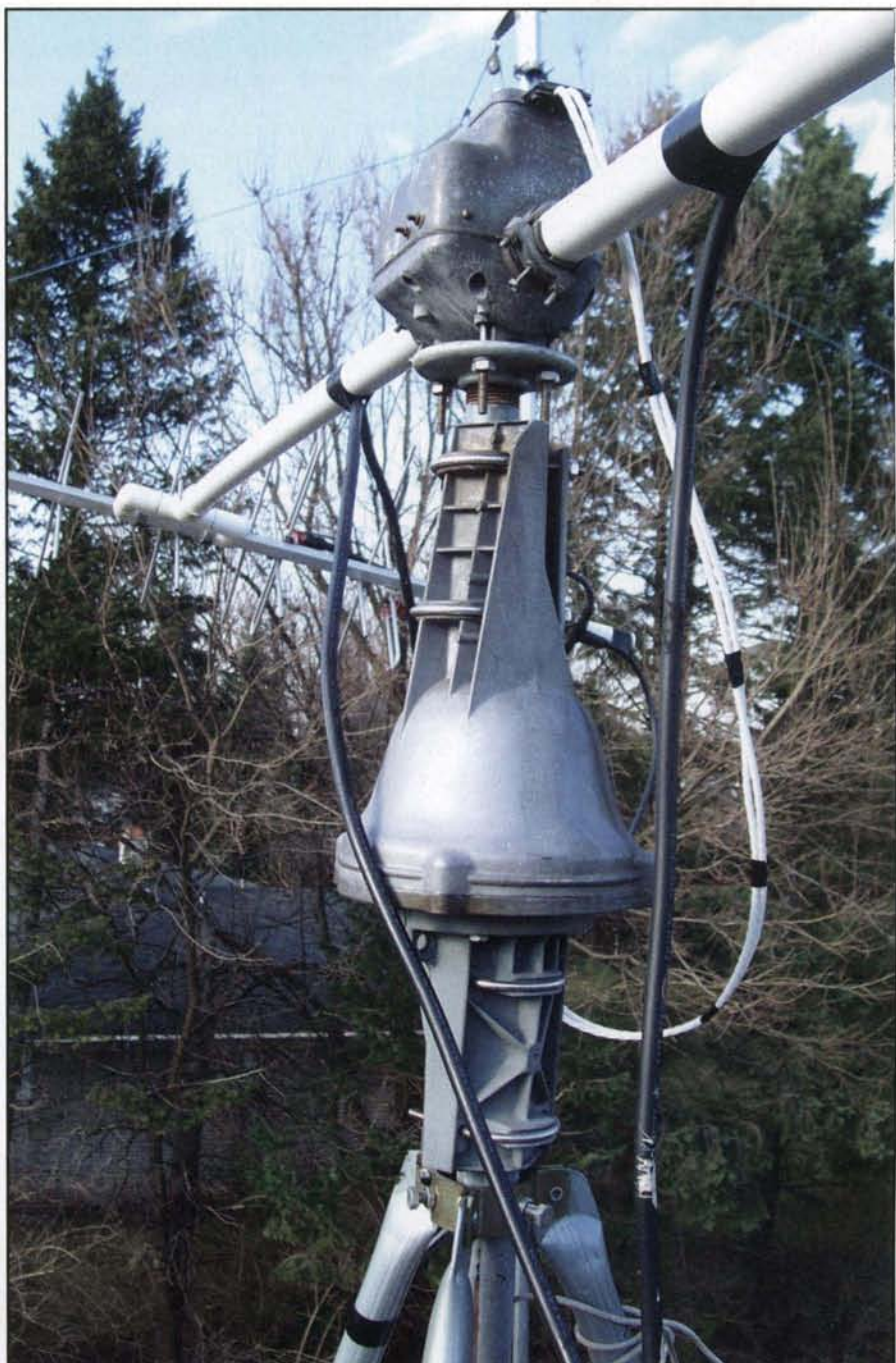
Photo 1. The two rotators showing the pipe and flange, 6-32 screw through the collar.
