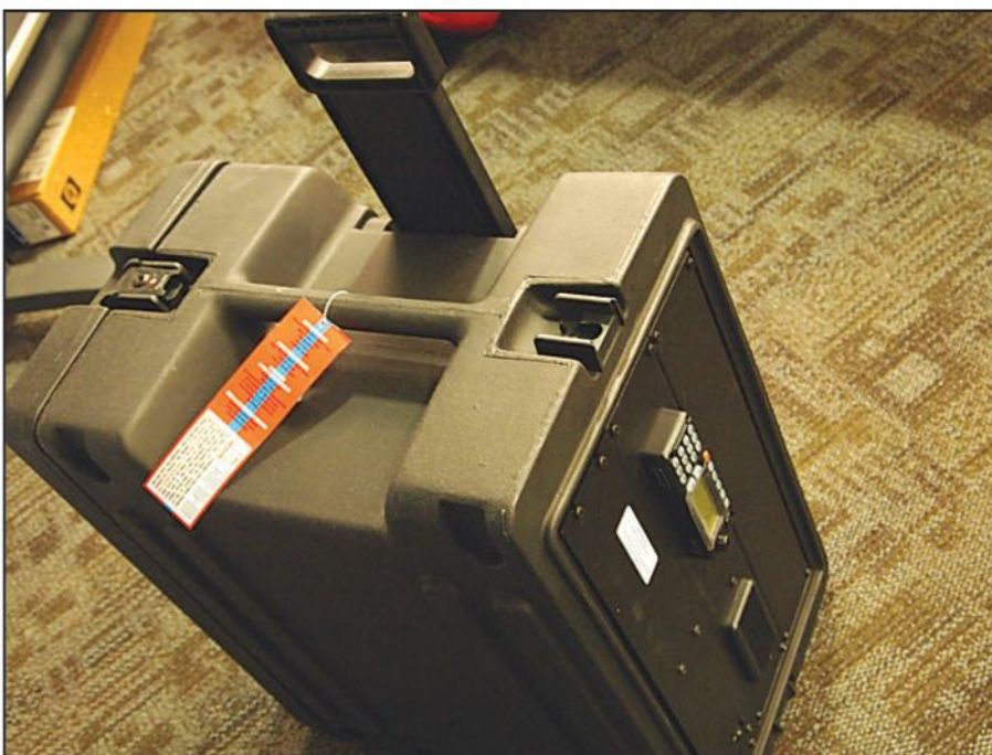
ID-1 deployable go-kit includes everything needed in the case except for the 1.2-GHz antenna, which is carried separately.
