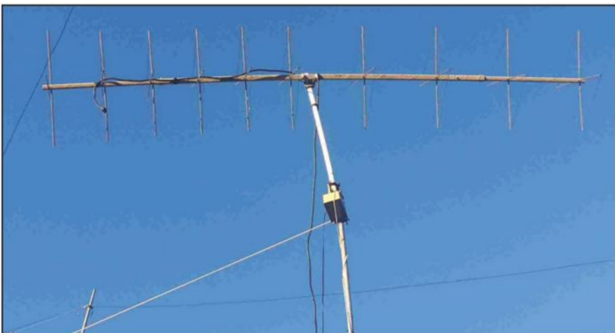
Photo 4. A 10-element 144-MHz antenna. (Photo courtesy N6CL)
