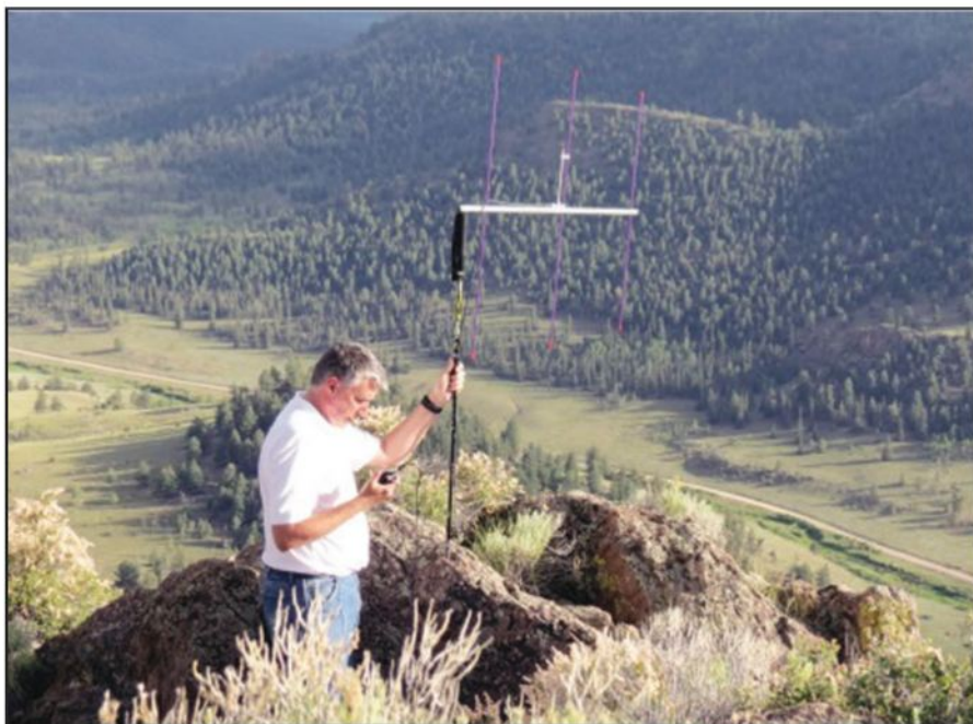
Figure 8. The Yagi antenna shown mounted on top of a trekking pole, using a 1/2-20 camera mount.
