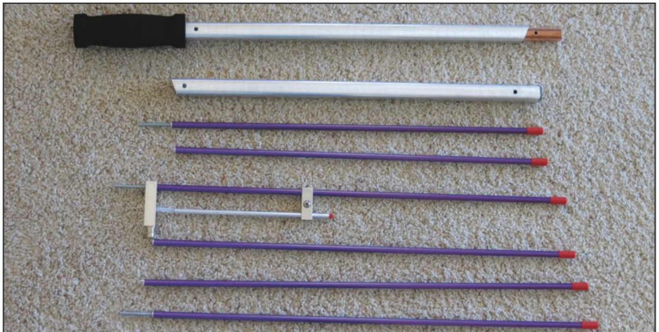
Figure 7. The 3-element Yagi antenna easily breaks down into eight pieces for transport.
