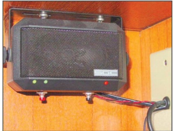
The SGC DSP speaker is amplified, with two levels of DSP.
