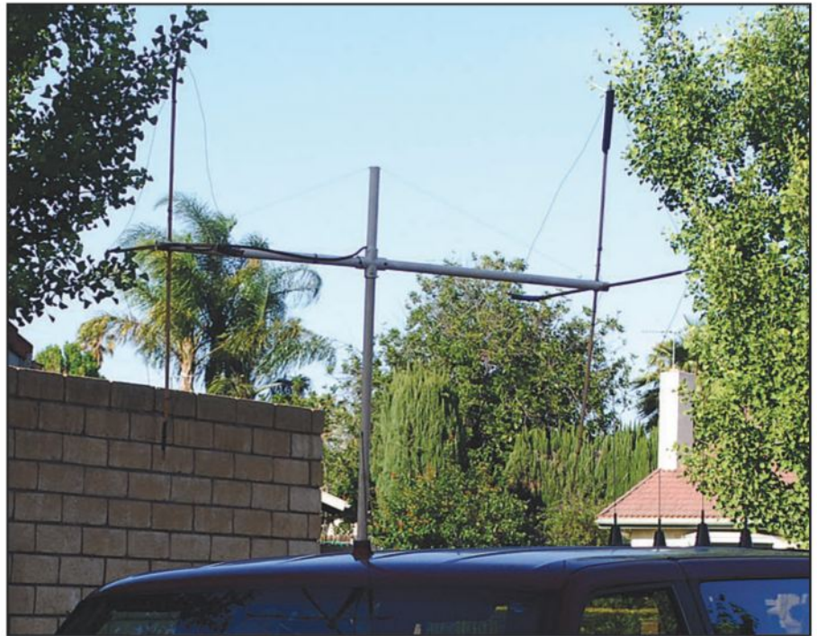
This shrunken quad has proven to be a sensitive and effective RDF antenna for 6 meters. The taped-up corners were field repairs for broken spreader tip dowels. Next time, fiberglass spreaders! (Photo by Joe Moell, KØOV)
