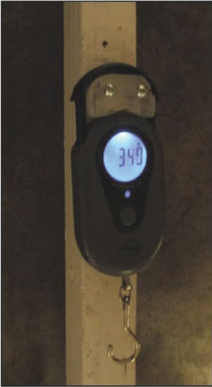
Photo 7. Fill scale used for precise measurement of the weight of the helium used to fill the balloons.
