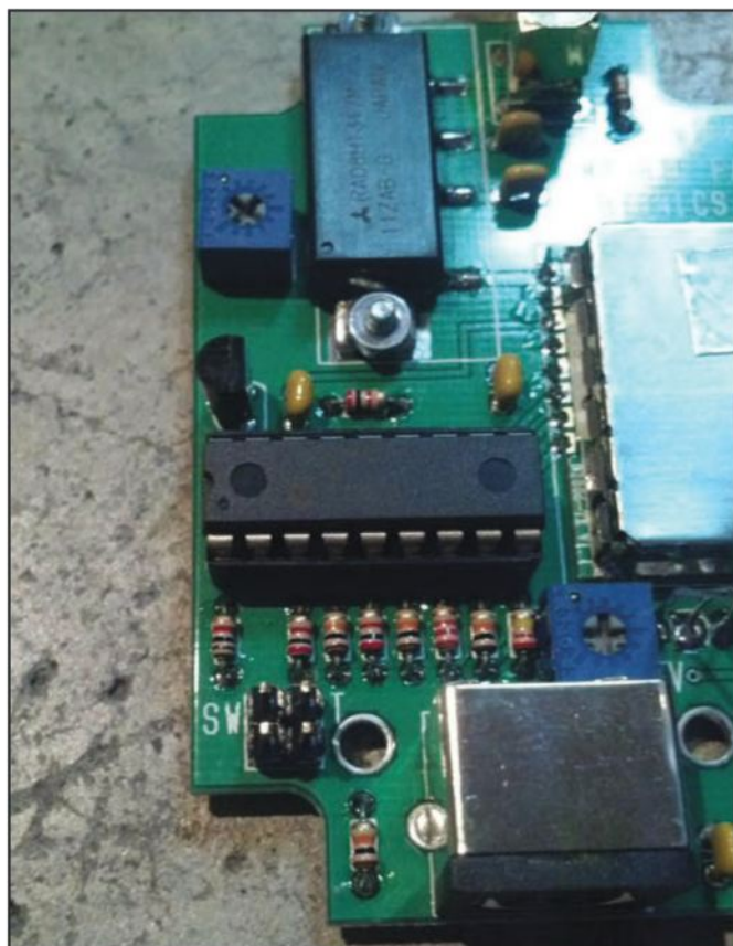
Photo 4. The MT-RTG beacon had standard jumper-pin pads that could be used to trigger the frequency switching.
