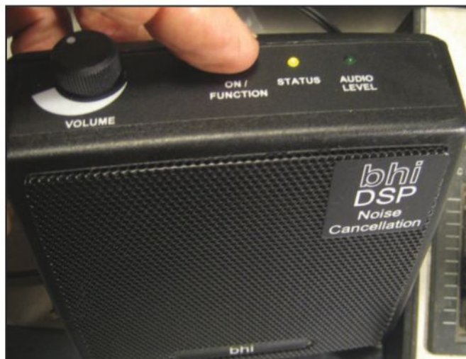
The bhi DSP speaker (available from Gap) amplified, with push-button level settings.
