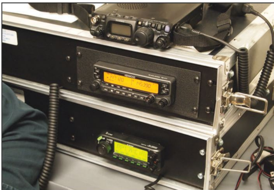
Close up of HF, analog, and digital transceivers, with ruggedized cases.
