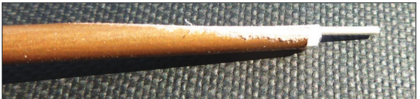
Photo C. Tapered coax side view.
