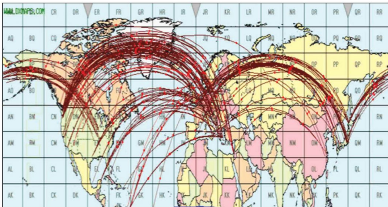
Figure 1. This figure shows northern 6-meter activity during 27–29 June 2012. To avoid covering up most of the map, this only shows contacts over paths of 8,800 km or more! (Map credit: < http://www.dxmaps.com >)
