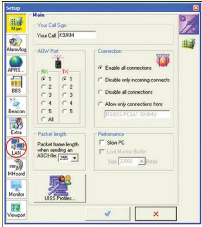
Figure 16. Setup of UISS with the red circle showing the LAN selection.
