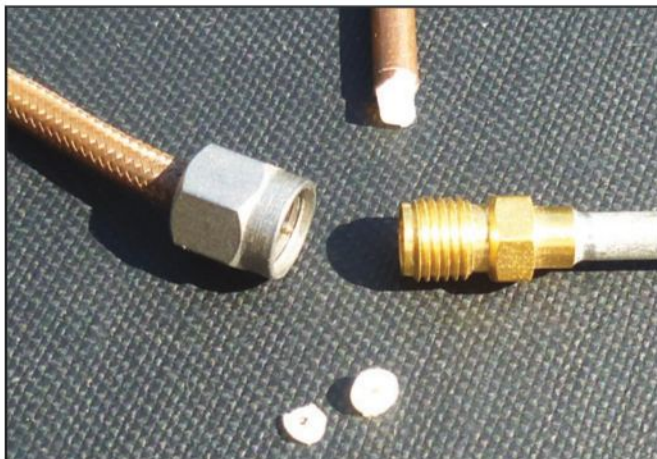
Photo E. Converting 50-ohm coax to 75-ohm coax.
