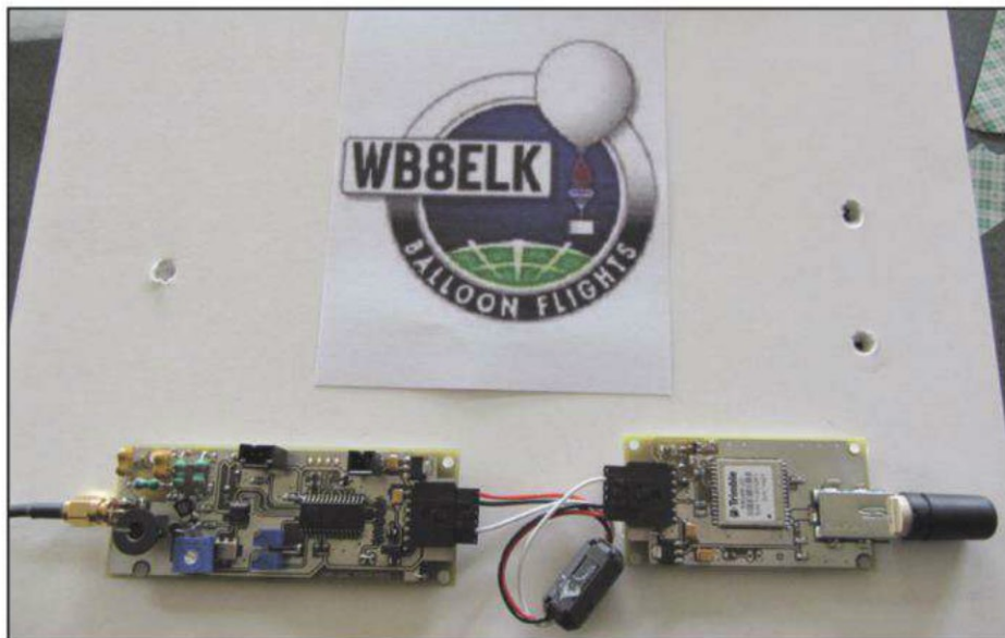
Photo 2. The 500-milliwatt 20-meter HF payload.
