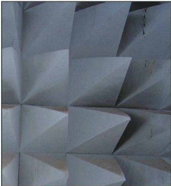
↑ Photo D. Tapered cones in an anechoic chamber.
