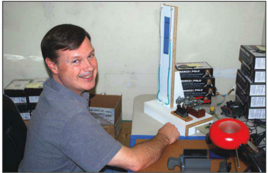
Tim Crabtree performs the pressure test on a Marco Polo dog tracking tag to verify that it will continue to work if Fido goes swimming. (All photos by Joe Moell, KØOV)
