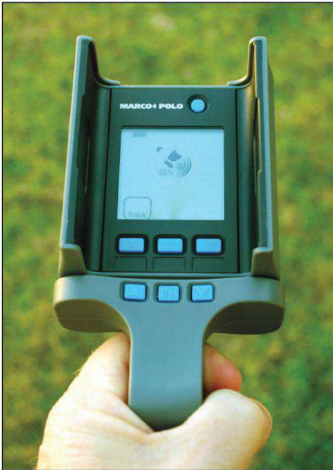
In addition to a directional arrowhead, the Marco Polo locator display shows signal strength as a percentage and by the number of curved bars.
