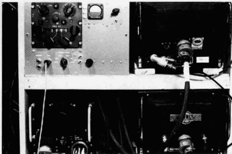
The ARC-58 system at KJ4KV. Clockwise from upper left: The control box (black panel), the transmitter, the receiver, and the PP-2352 inverter. The gray panel at upper left contains audio input and output and interconnect wiring, metering, and other external circuits.
