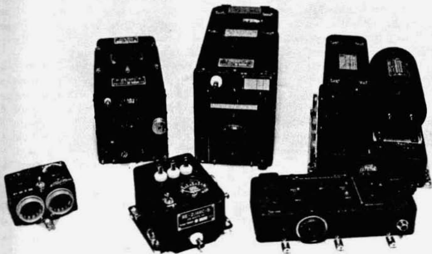
Command Sets -- Top row (L to R): AN/ARC-5 receiver; transmitter, and modulator. Bottom: C-30A/ARC-5 control box for up to four transmitters, one of which is VHF; RE-2 antenna relay; and C-38 control box for up to three receivers and an ARR-2 navigation set. Note covers over unused controls on C-38; this was a common way to adapt a control box to a specific installation.
