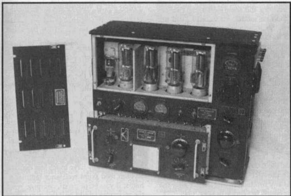
The BC-375. The tuning unit has been pulled part way out. Operating with the tube compartment cover removed as shown will definitely help you keep warm on a chilly 'midwatch' in the shack!
