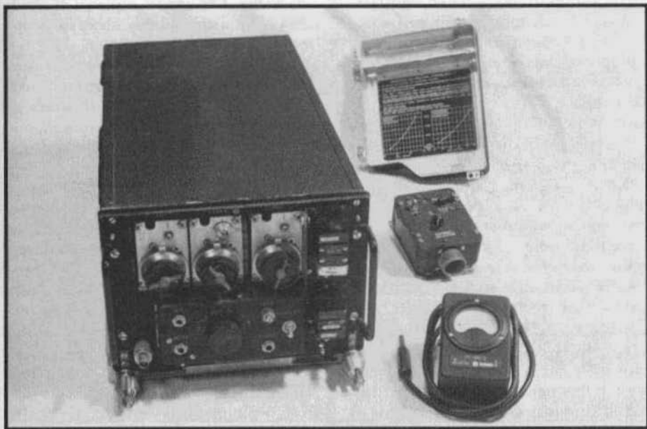
The ARC-1 transceiver. At right are the tuning tool, TS-80 meter used for tune up, C-45/ARC-1 control box, and front panel cover with tuning curves.
