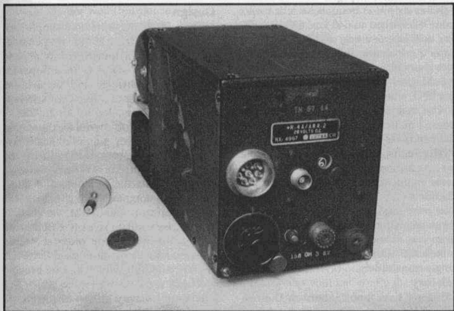
The ARR-2 receiver. The knob can be attached to the threaded bushing near the center of the panel for local channel selection.
