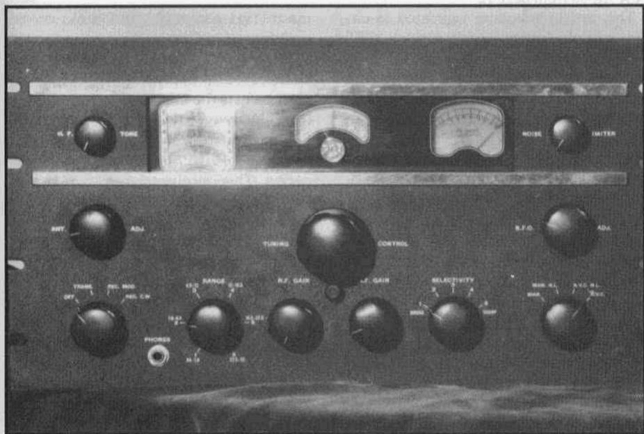
The original AR-88. Note the large RF and AF gain control knobs below the tuning knob.
