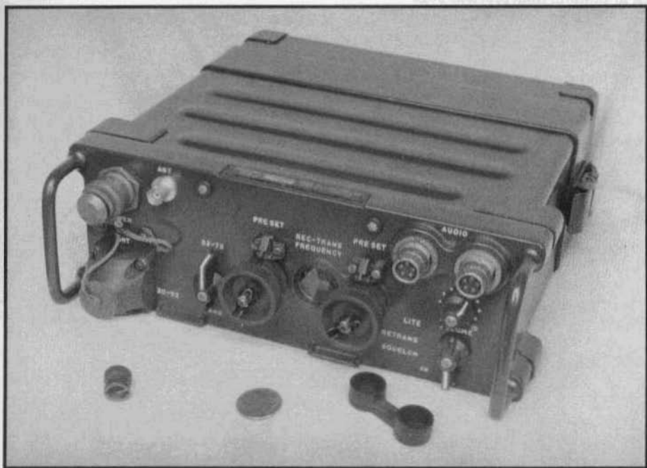
RT-505/PRC-25. The BNC jack cover and AUDIO jack dust cover would normally be anchored by lanyards. Latches near the rear hold the battery case, which (because the set is transistorized) is a fraction the size of those for earlier portable radios.
