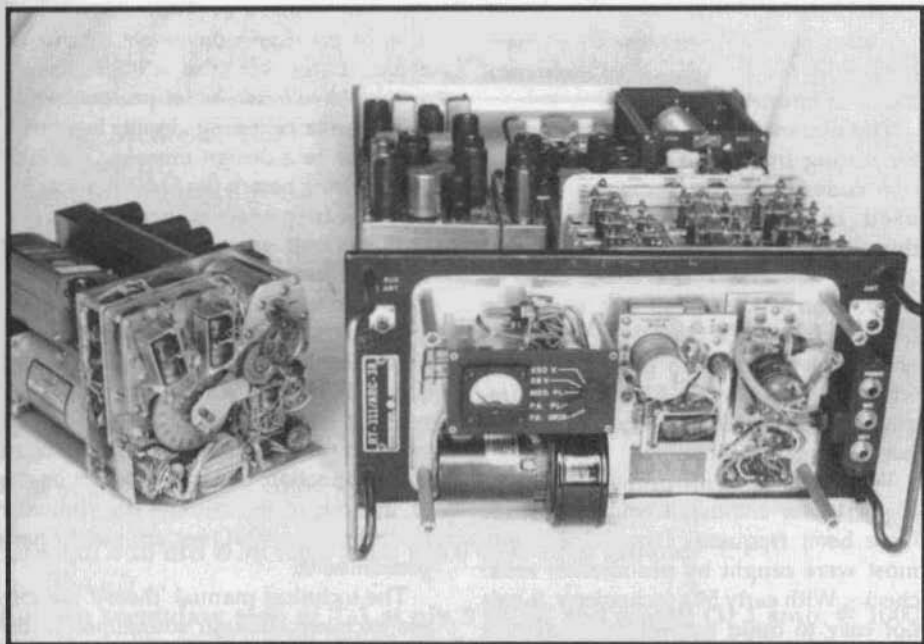
The ARC-38 with the covers off. The tuner module is at the right front, the PA assembly at the rear. The SMO is out of the set, at the left.
