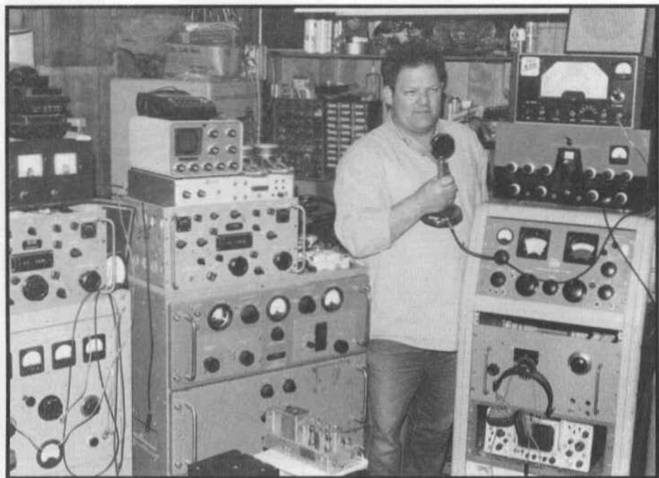
Don Spreeman, WA9ZOR, Kaukauna, Wisconsin, with some of his gear. On 160 he uses the T-368 with a SP-600 or R-390. His antenna on 160 is a 85 ft. base-loaded vertical.
