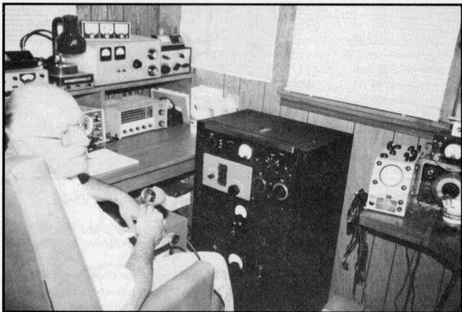
Charlie Carpenter, W5TOP, operating his 813 homebrew rig. Note the T-368 exciter unit built into the RF deck. Also shown (above and to the left of the 813 rig) is a 3-500Z homebrew amp for SSB.
