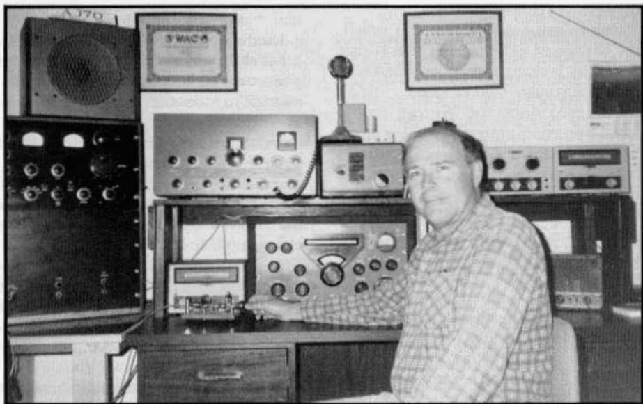
Dave Mills, AJ7O, in his shack. From the left we see Dave's 813 homebrew CW transmitter, HG-10 vfo, Viking II and R-388. Above the R-388 is a T-368 exciter unit, mounted in a cabinet, that Dave uses with his homebrew rig as well as the Viking II.
