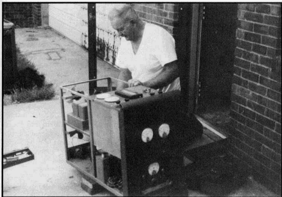
Russ removing transformers from the Johnson KW before loading it in his van.
