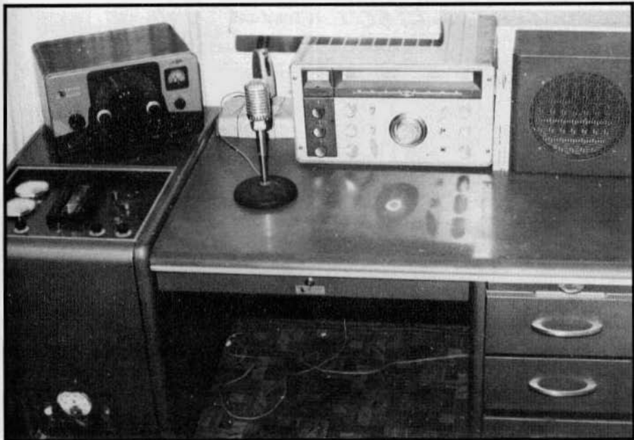
E.F. Johnson's response to the Collins KW-1, the Desk Kilowatt. On the left is the Ranger exciter and next to it is a National NC-300 receiver.
