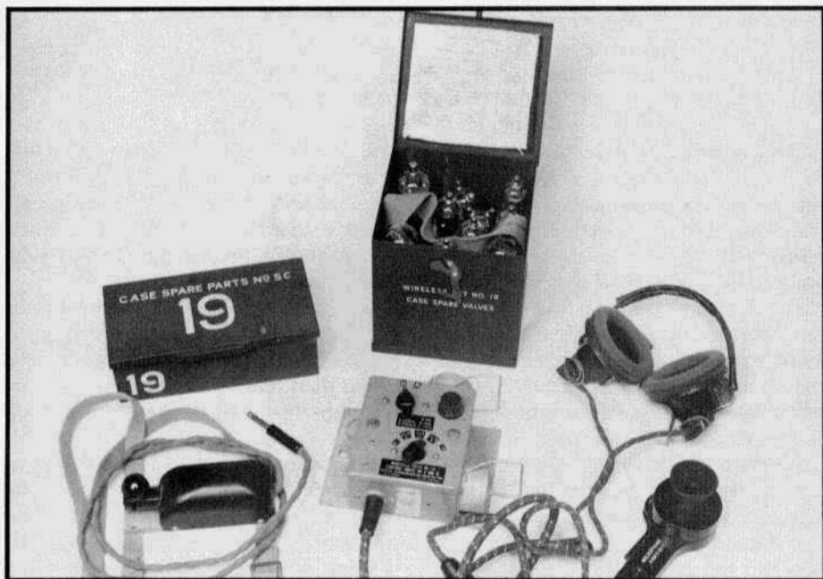
No. 19 accessories. Clockwise from lower right: microphone; key; spare parts box containing fuses, dynamotor brushes, lamps, and space for the key; spare tubes box; headphones. A typical control box is at the center.
