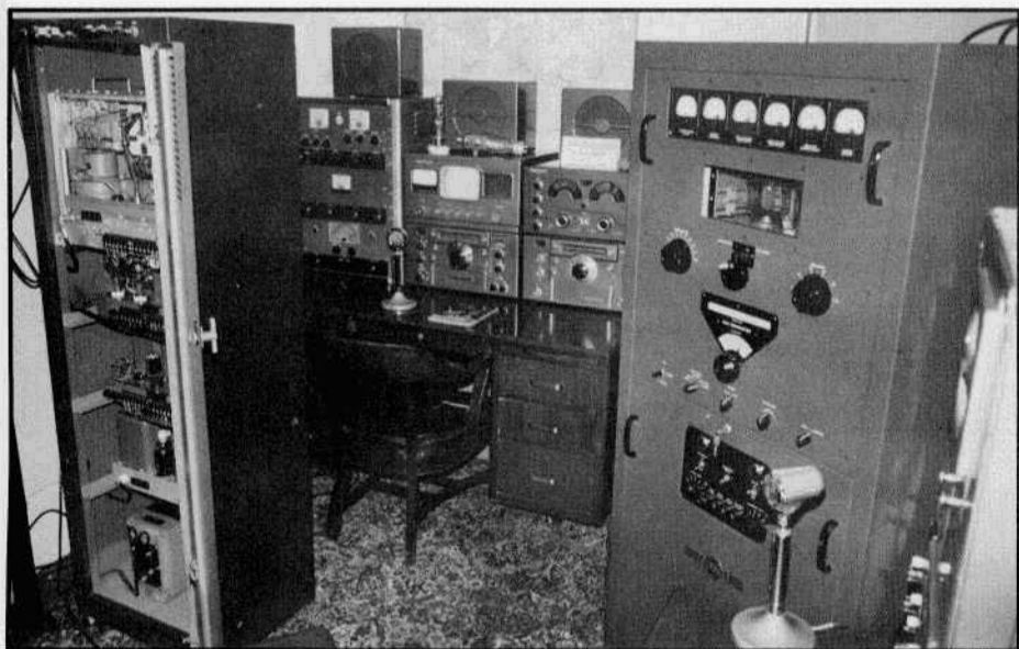
The shack of Sam Thompson, W6HDU , showing his KW-1 on the right, the rear of his 30K-1 on the left and operating position in the center. On the left end of the desk is a Globe King 500B. Next to the Globe King are two HRO-60's on the bottom with a Hallicrafters TV-7 Videometer TV (1951, in operation) and a NC-183D above.
