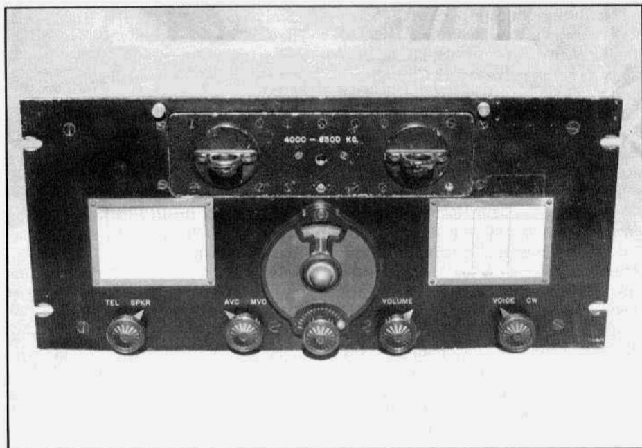
Figure 3. The AGU receiver showing its unit plug-in coil installed. The AGU was also known as the RHQ in commercial applications.
