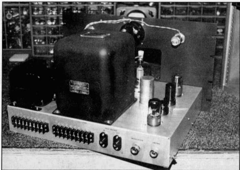
Rear view of modulator showing modulation transformer in middle, speech amp on right and power supply on left.
