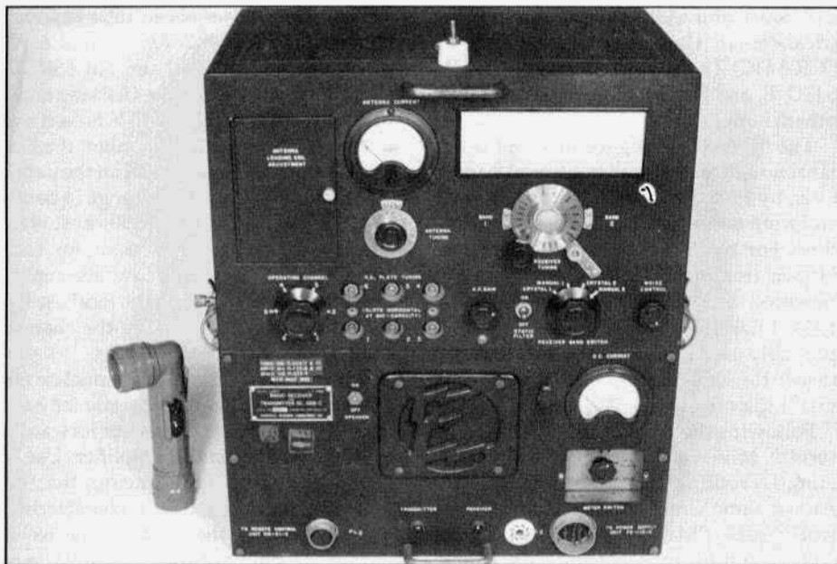
The BC-669 transmitter-receiver. The final amplifier tune up holes and meter switch access would normally be covered by plates. Hinged door at upper left allows adjusting taps on the series loading coil; the tank coil taps are reached through a hinged lid on top of the set. The feed-through insulator at top center is the antenna connection. Hallicrafters sets have an 'h' in the speaker bezel.
