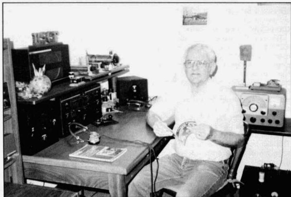
Vane Gildersleeve, K5CF, with some of his vintage gear which includes a RME -70, homebrew 6L6 rig, a National SW-3 and a TNT transmitter. He uses the TNT and SW-3 for AWA contests. Also shown is a Ranger II and a Drake R-4B.
