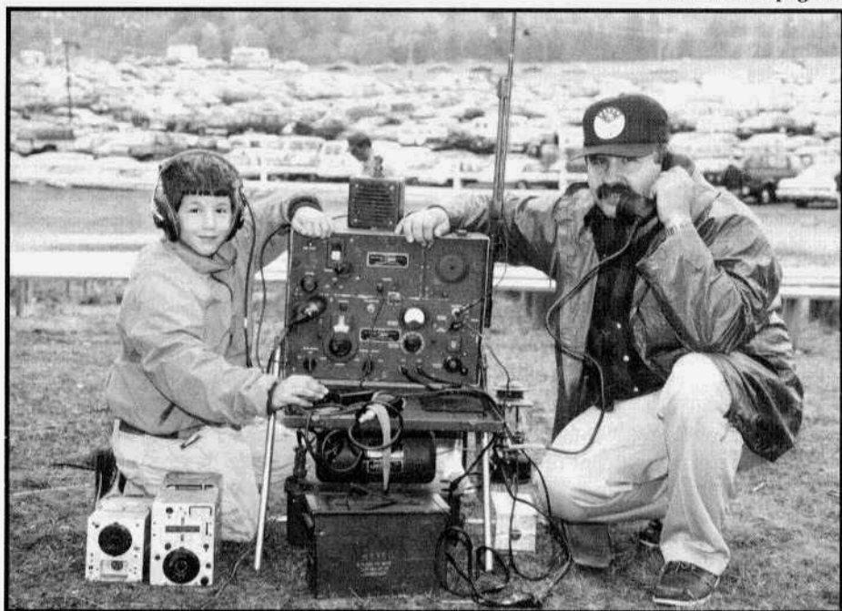
Ben, KA1YKG, and his dad Chris, AJ1G, operating a BC-654 field set on 3885 Khz into an 8' loaded whip with radials on the ground.
