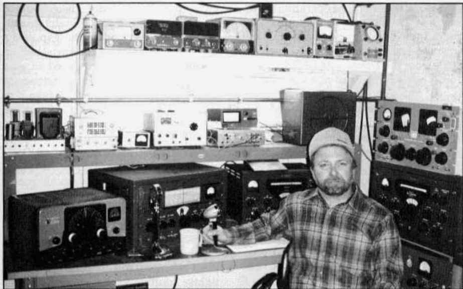
Bill Owen, KF0IE, says most of his activity is on ten meters. One of the transmitters he uses is the Stancor ST-203 that's located on the shelf above the Ranger.
