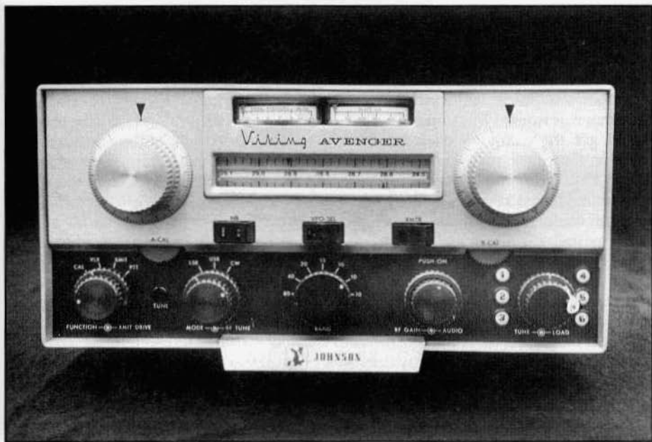
Front panel of the Avenger. It's 5 inches high and 11 inches wide.
