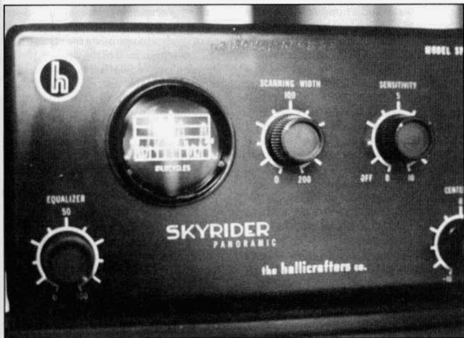
Close-up of SP-44 front panel while in operation. Note the waveforms on the CRT.
