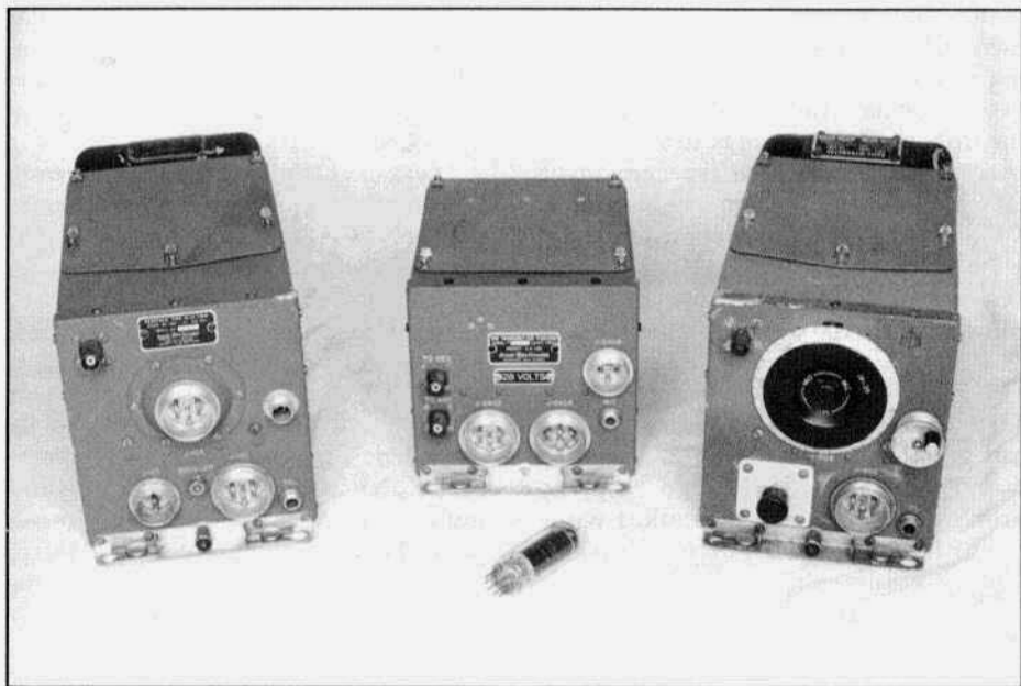
Some ARC type 12 sets. Left to right: R-15 receiver, T-13A transmitter and R-19 receiver modified as described in the text. This transmitter uses 5763's as oscillator, multiplier, final, and modulator; earlier models used 6AQ5's and delivered about 2 watts of output. The transmitter gets plate power from the receiver dynamotor.
