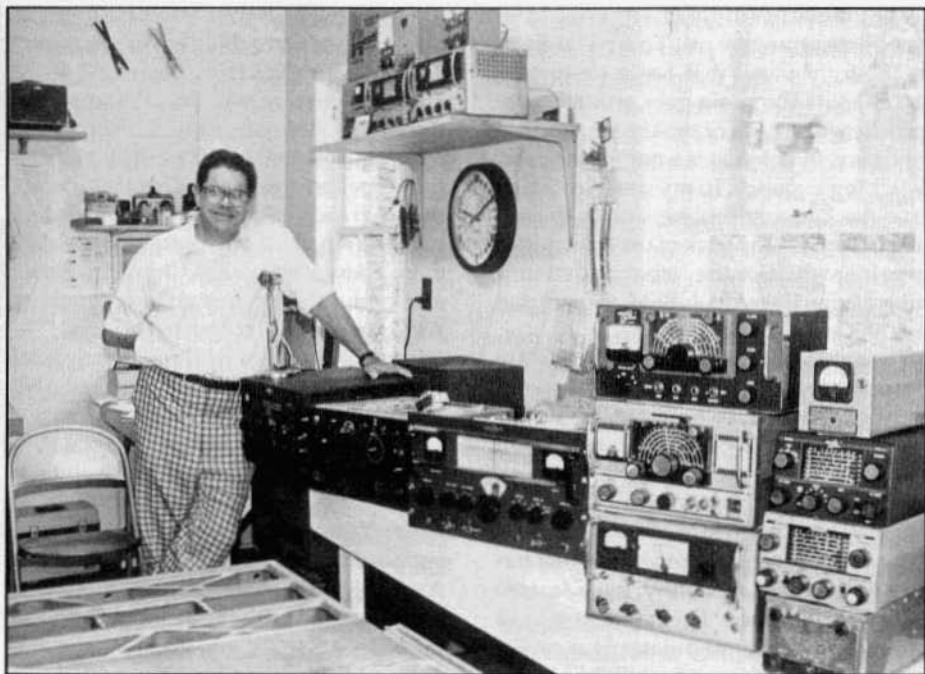
Lea Salter, KN4JW, in his workshop/hamshack. The Multi-Elmac gear is in two stacks on the right of the photo. On the top of the left stack is the AF-68 transmitter, below it is the AF-67 and on the bottom is the A-54 transmitter. The right stack consists of (from the top down) the PSR-612 power supply, the PMR-8 receiver, PMR-7A receiver and PMR6A receiver.
