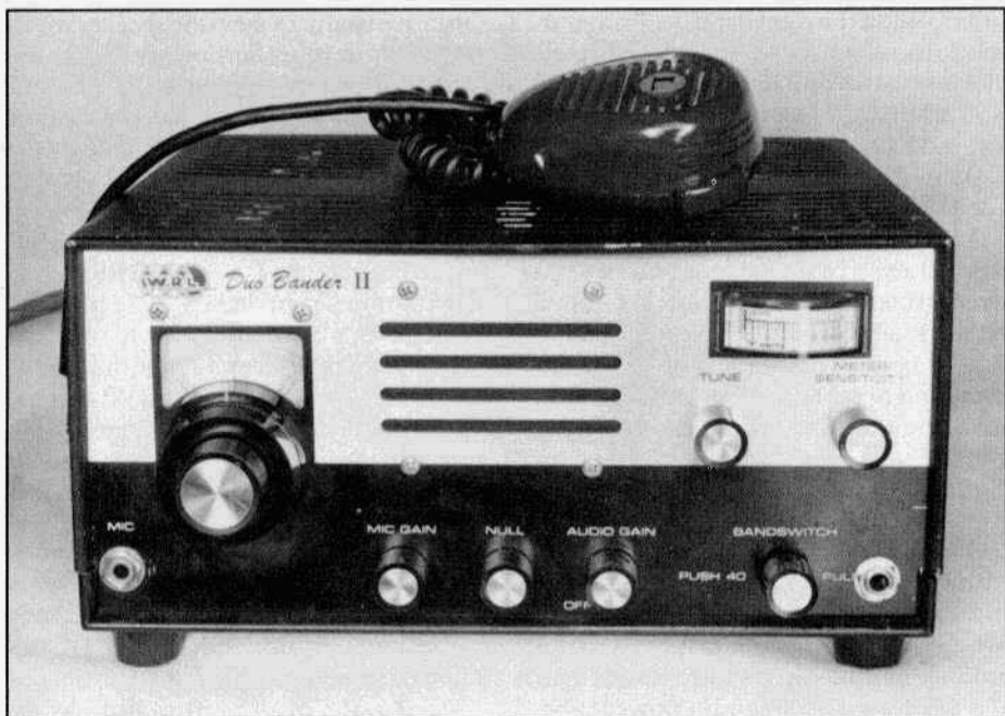
The WRL Duo-Bander II. Headphone jack at the right was installed in a hole drilled by the previous owner.
