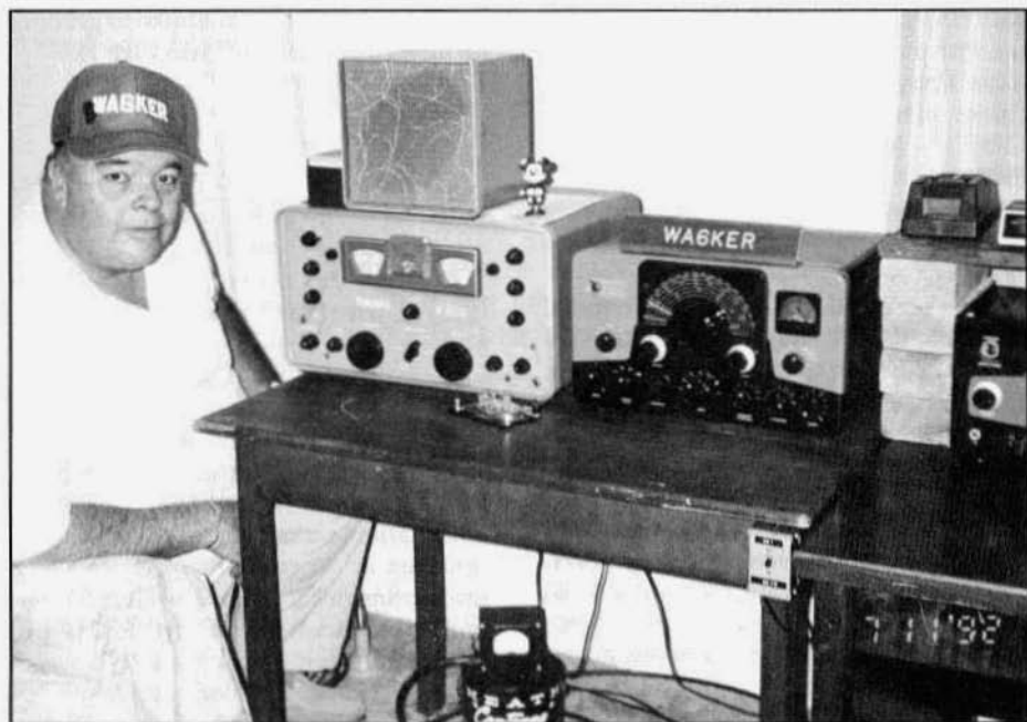
Bob Braeger, WA6KER, with a classic vintage station; Johnson Ranger I and Hammarlund HQ-160.
