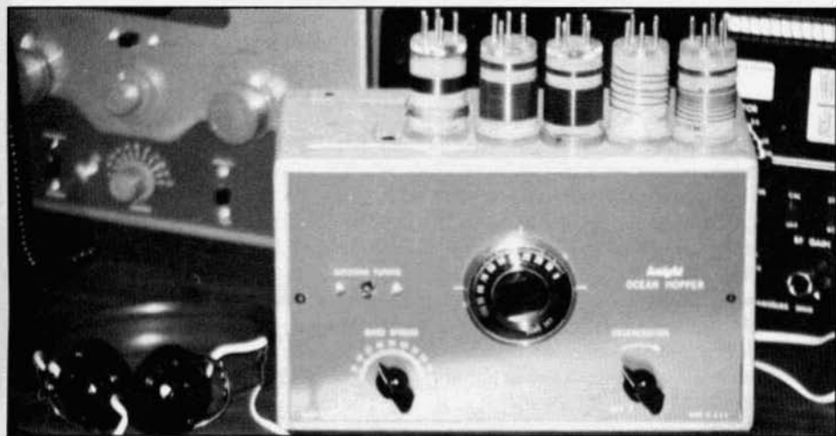
The restored Ocean Hopper with a complete set of coils and headphones.
