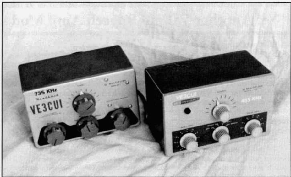
The modified QF-1 on the left and the stock HD-11 on the right.
