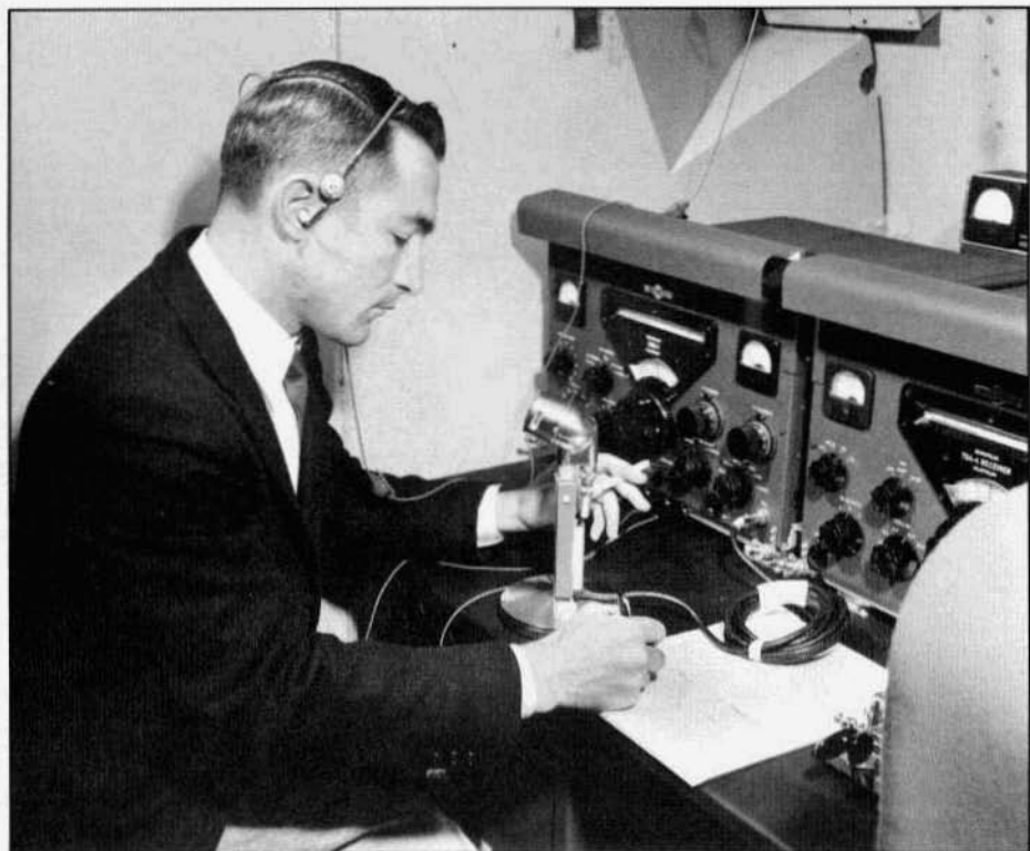
A 75A-4 and KWS-1 aboard an aircraft during the period when the airforce was evaluating SSB for military use. Photo courtesy of Harry Snyder, WØRN.
