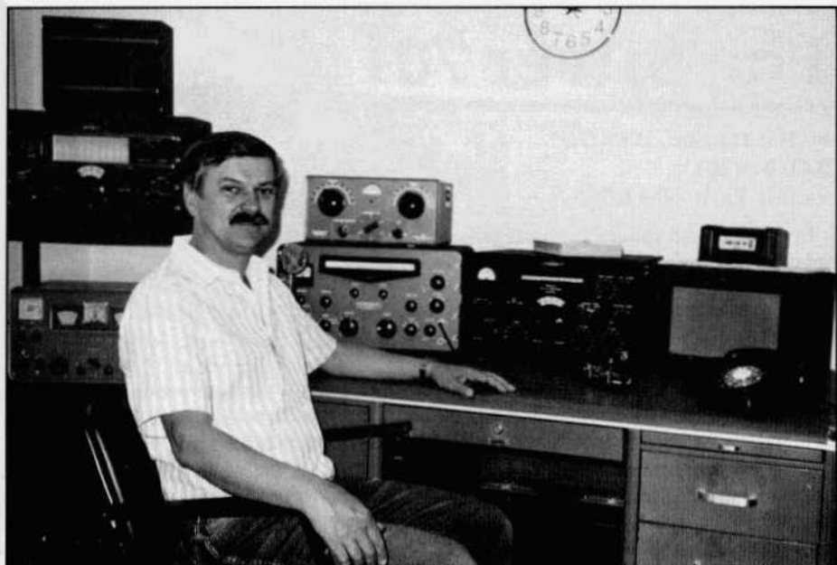
Joe Eide, KB9R, with a vintage SSB station. The transmitter is a Gonset GSB-100 and the receiver is a 75A-4. The tuner sitting on the GSB-100 is a Millen 92200.
