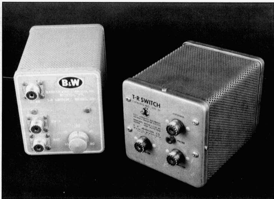
Electronic TR switches, the B&W model 381 on the left and the E.F. Johnson 250-39 on the right.
