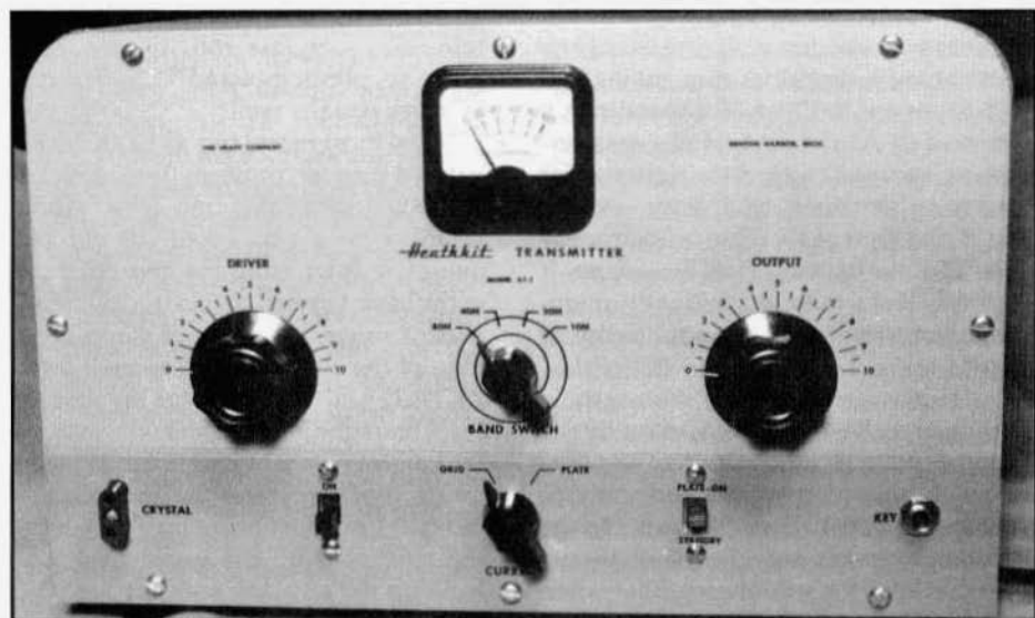
Front panel of the rebuilt AT-1.
