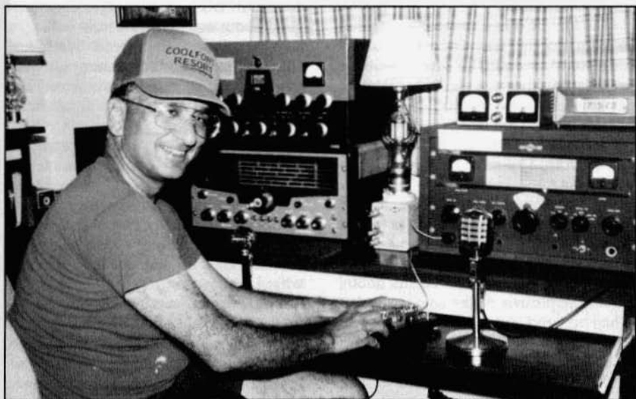
Tom Marcellino, W3BYM, with his vintage station. On the left a Viking II sits on a Hallicrafters SX-101A. The transmitter on the right is a Collins 32V-1. The mic in front of it is an Electrovoice 911. The mic with the Viking II is an Astatic JT-30.
