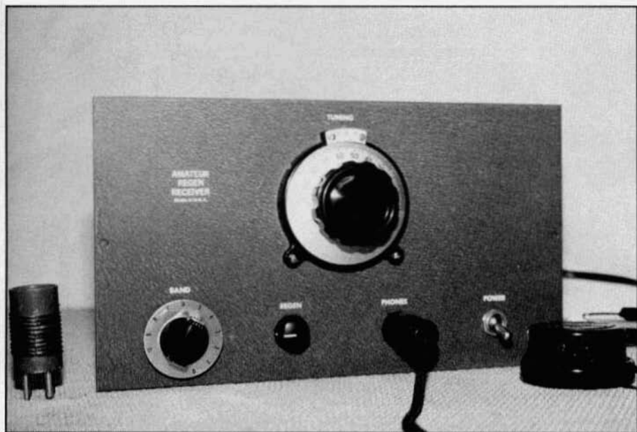
Front panel of regen. receiver with headphones and coil.
