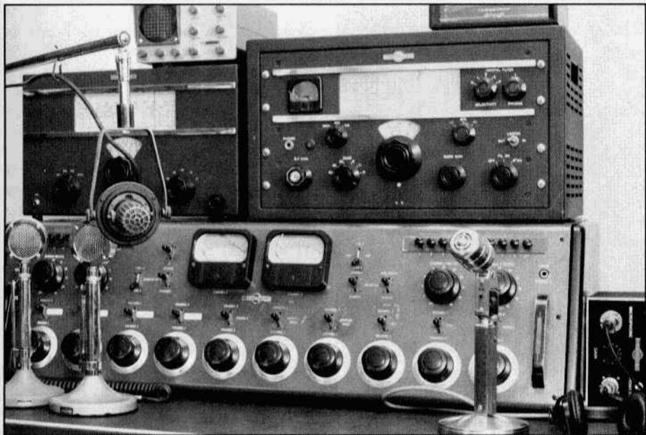
Sitting on the Collins 212A-1 console is a 310A-1 exciter and a 75A-1 receiver. Out of the picture, to the right is a rack containing the speech processing equipment.
