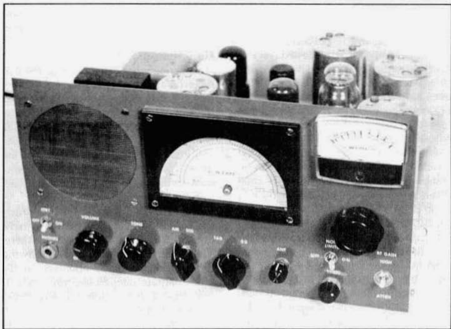
Figure 1. The nine-tube, band-switching superhet tunes the 160 and 80 meter bands. All controls are marked with Dri-Transfer labels.
