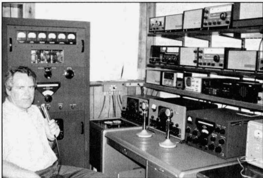
Jim Jorgensen, K9RJ, with some of his vintage equipment which includes a Collins KW-1 and Johnson Desk KW. Sitting on the desk is a Ranger, a Valiant and a 75A-4.
