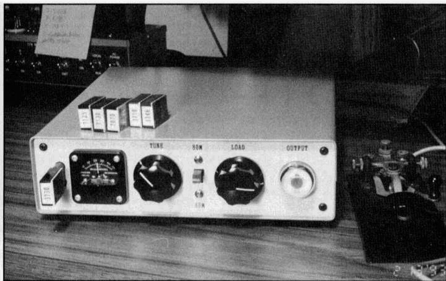
The two-tube xmtr was built into a Ten Tec Constructo Series enclosure. Total cost was $75.
