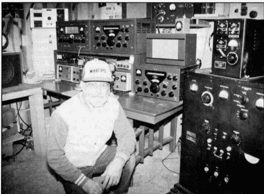
Art Rideout, WA6IPD, with his vintage gear. The transmitter on the right is a BC-610.
