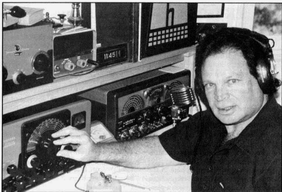
Harvey Laidman, N6HL, at his operating position. The vintage gear shown includes a Johnson Ranger I transmitter, Hallicrafters SX-100 receiver, Johnson Matchbox and Hallicrafters TO keyer.
