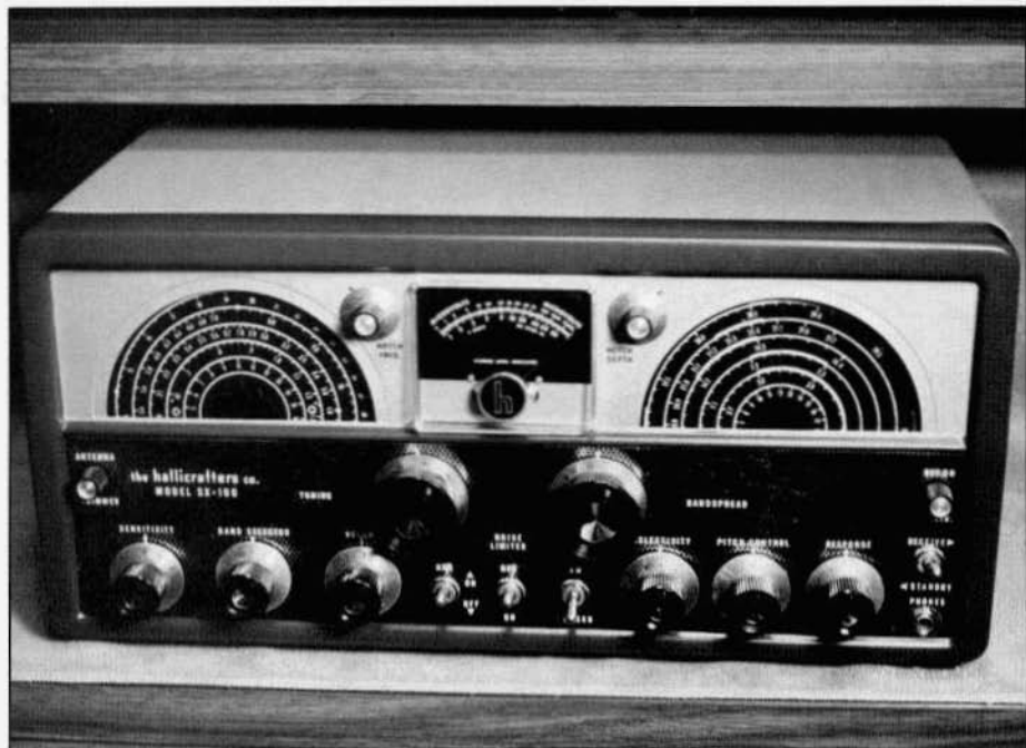
The restored Hallicrafters SX-100. This general coverage, 14 tube receiver sold for $295 during the years it was manufactured - 1955-1961.
