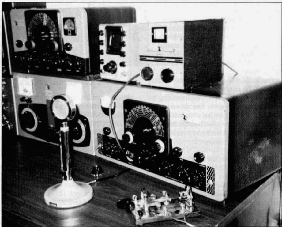
Johnson Viking 122 VFO modified for NBFM connected to a Valiant transmitter.
