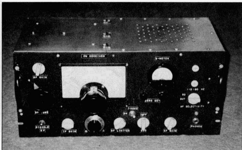
A homebrew receiver designed to tune only the 80-meter CW band. The power supply is on a separate chassis.
