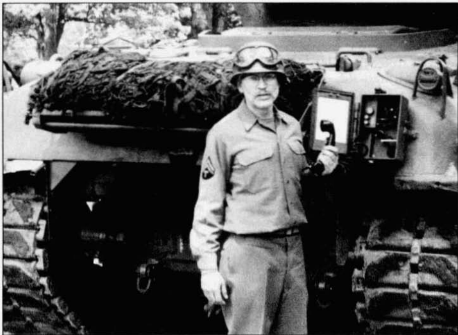
The author talking to the crew of a fully restored 1945 M4A1E2 "Heavy Sherman" tank on an original BC-1360 armored external control box. This is a heavy version of the M4 "Sherman" tank with the larger 76mm gun, large turret and double wide tracks. The tank gets 4/10 mile per gallon of gasoline.
