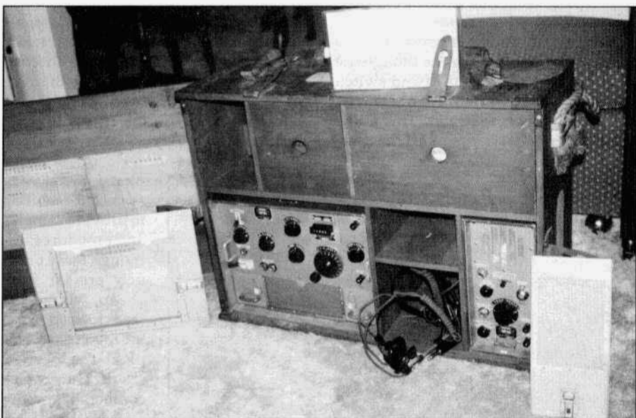
Joe Schroeder, W9JUV, recently acquired this very unusual Japanese WW II receiver complete with its shipping crate that also contains earphones, spare tubes, full set of plug-in crystals (300 kcs - 6 Mcs), charts, etc. He would like to hear from anyone who has information on this set. His address is Box 406, Glenview, IL 60025-0406.
