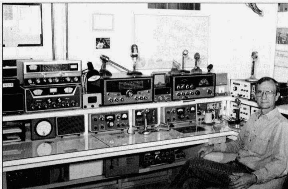
Another beautiful, well-organized hamshack. James Buchanan, K8WPI, says this is operating position #3; his favorite and most used position. He says the 'prize' of his station is the 1930's "antenna field strength" meter, which has been mounted on a mahogany face plate, located far lower left.
